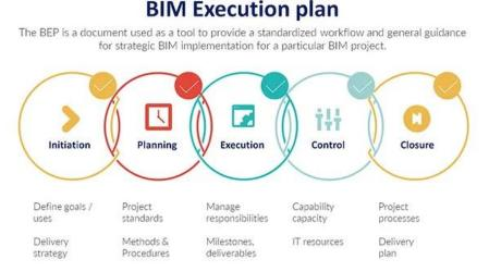
A BIM Execution Plan should be created during the early design phases of any project and amended or refined as necessary through implementation and beyond. It should define scope, process flow, BIM tasks performed during implementation as well as any information exchange between parties involved and define infrastructure needed for project implementation. The BIM Execution Plan has been acknowledged as a living document that usually includes:
