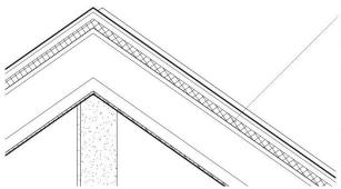
Ceramic roof tile Wooden batten 30x50 30 mm Wooden counter batten 40x60 40 mm Waterproofing 1,5 mm Wood formwork 24 mm Thermal insulation /d,max = 0,037 W/m.K + rafters 1 m 200 mm Thermal insulation /d,max = 0,037 W/m.K 60 mm Plaster profile UD, 2 x CD Vapour barrier 1 mm Gypsum Plasterboard 12,5 mm
