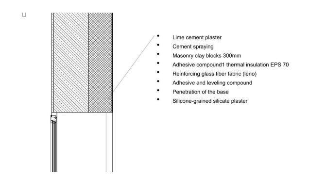
Detail of the external wall under terrain
