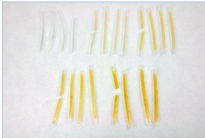
Figure 5 – Gradual discoloration of a PE film when exposed to UV radiation at various time intervals. Samples are arranged from upper left to lower right with the former having an exposure time of one week and the latter having an exposure time of one year. 17
