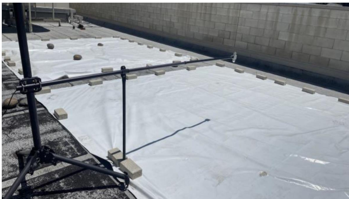
Figure 7 – Experimental setup of albedometer and candidate 4 m x 4 m PE sheets secured with grey bricks along their perimeter on the roof of building 41A on the Cal Poly SLO campus. In the sample on the left, 3 extra stones were temporarily placed on it while recording albedo measurements if the conditions were too windy and causing the sheet to flutter.
