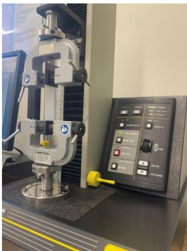
Figure 9 – Instron Micro Series 55MT2 tensile tester used in testing mechanical properties of candidate albedo materials before and after accelerated UV exposure.
