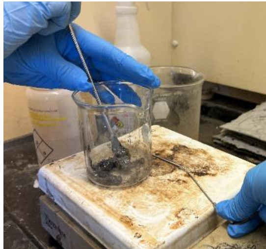
Figure 24. The 65 vol% mixture was harder to melt because of its clay-like nature associated with the higher vol% loading.
