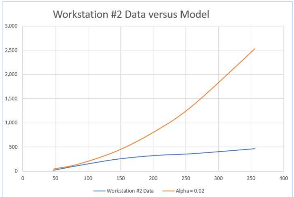
Figure 118: HRR (kW) over time (s) for workstation #2 data and the \alpha t^2 model with the \alpha value of 0.02 kW/s 2 used. Ordinate is HRR (kW), and abscissa is time (s).
