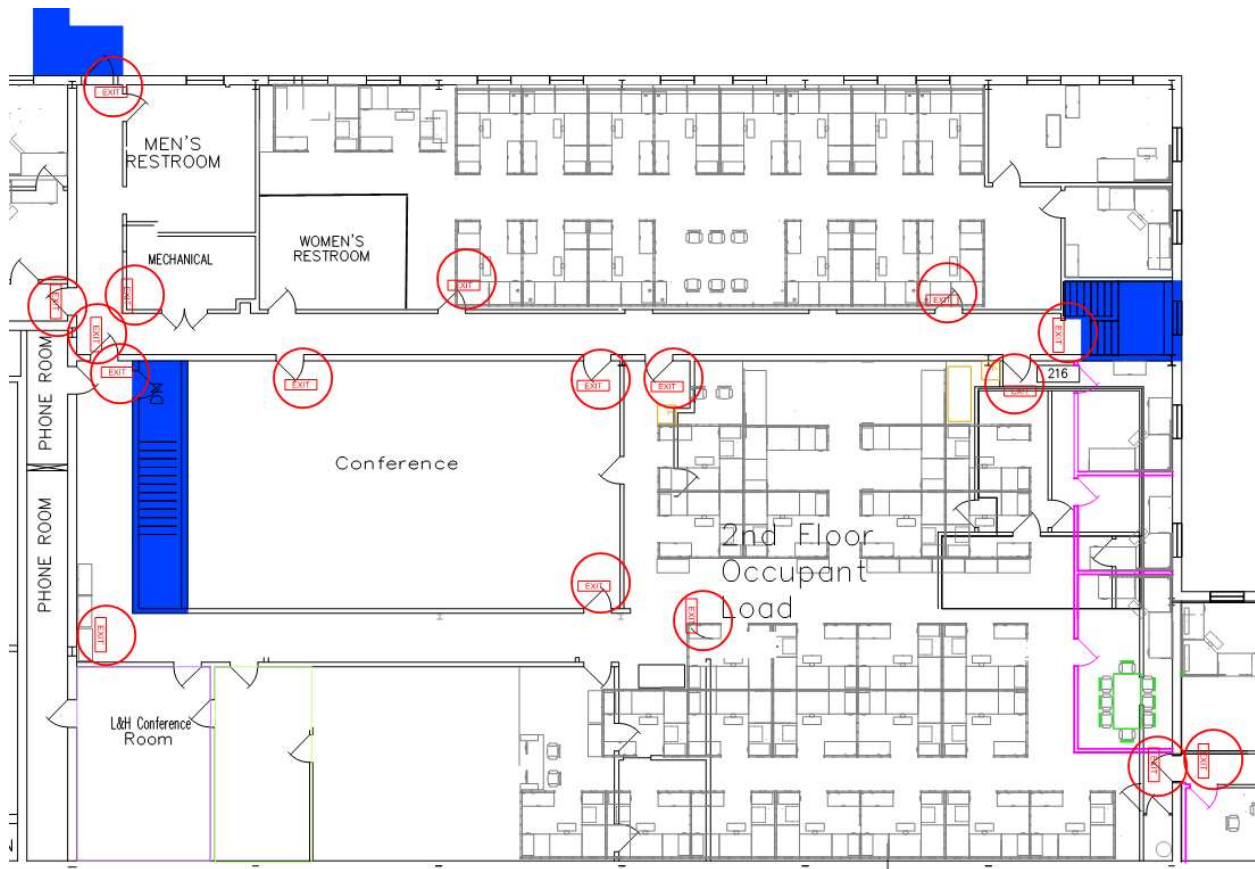
Figure 99: Exit sign placement for a portion of the 2nd floor office area.
