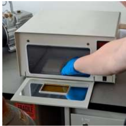
Figure 27. Loading platform in crosslinker.
