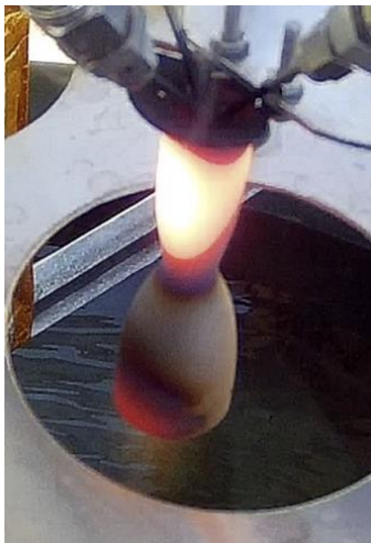
Figure 2.3-2 Stellar Exploration 1 lb f engine
