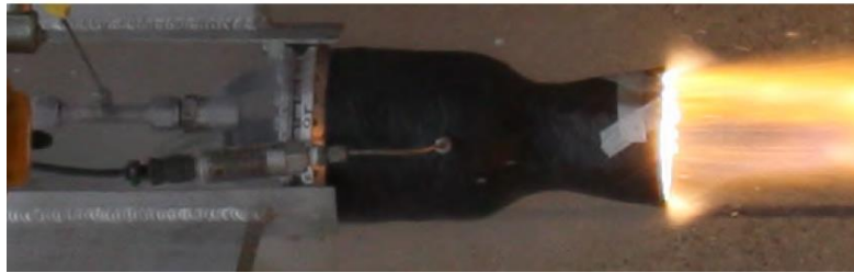
Figure 2.3-1 Purdue rocket engine CAD asem. and test fire [10]
