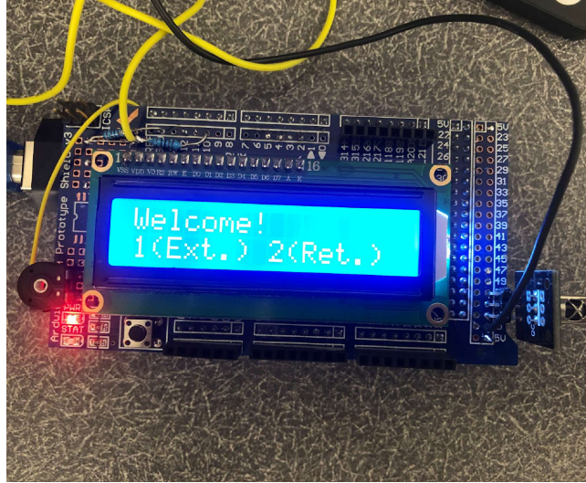
Figure 3.12: Soldered Prototype Shield Circuit.
