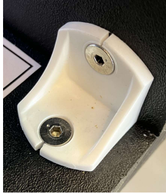
Figure 4.3: Cracked corner bracket.
