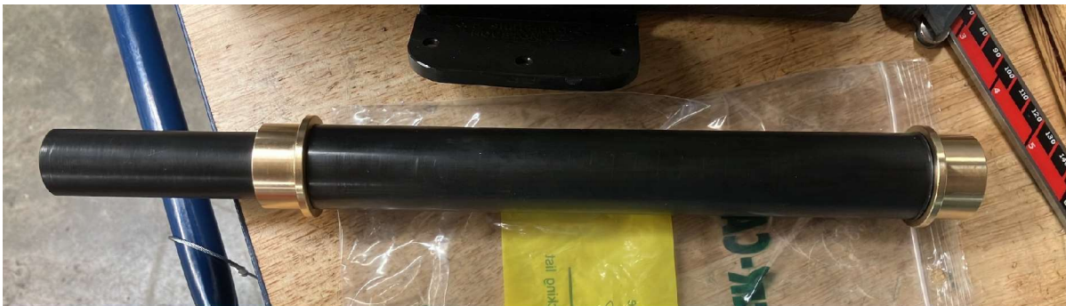
Figure 3.2: Shaft after finished on the lathe with bushings on.
