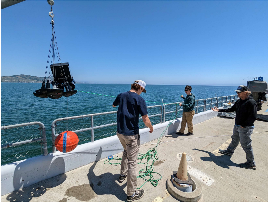
Figure 4.8: Lowering of the system for the submerged test.
