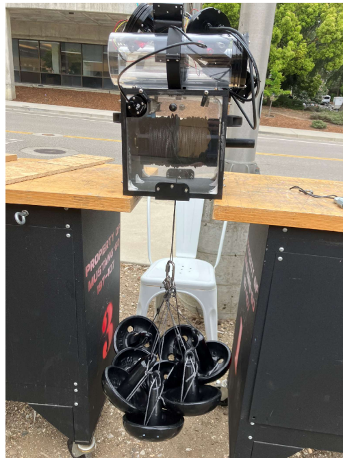
Figure 4.2: System set-up for shock loading test.
