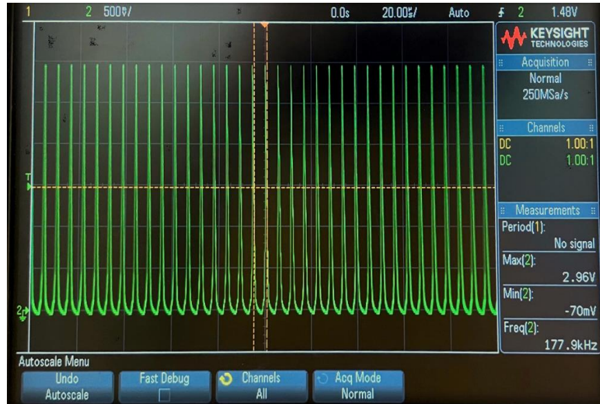
Figure 27. Dual Load Cell Noise Scope Capture
