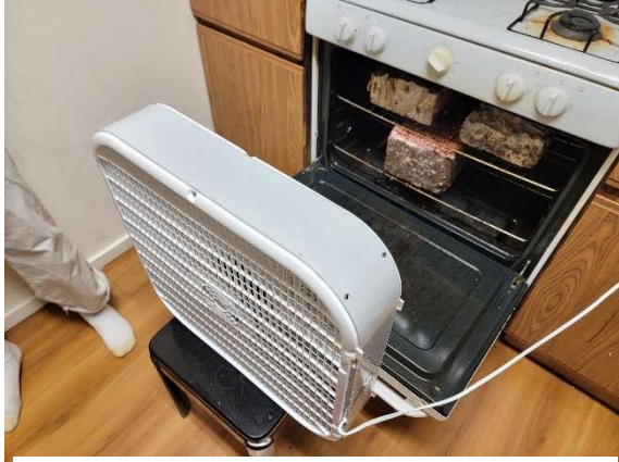
Figure 6 Box Fan Dehydrating Bricks in Warm Oven
