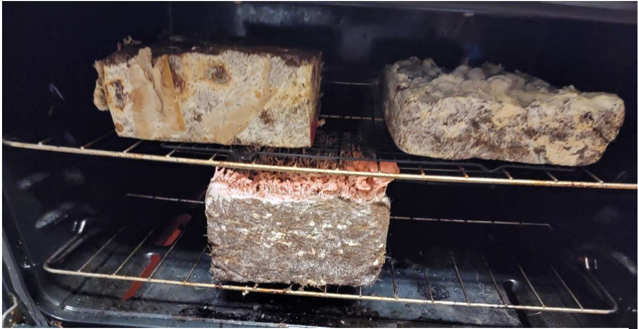
Figure 12 Three Mycelium Bricks in the Oven, Dehydrating
