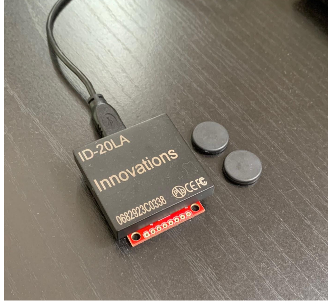
Fig. 5: RFID Scanner- ID-20LA (125 kHz) and RFID Tags
