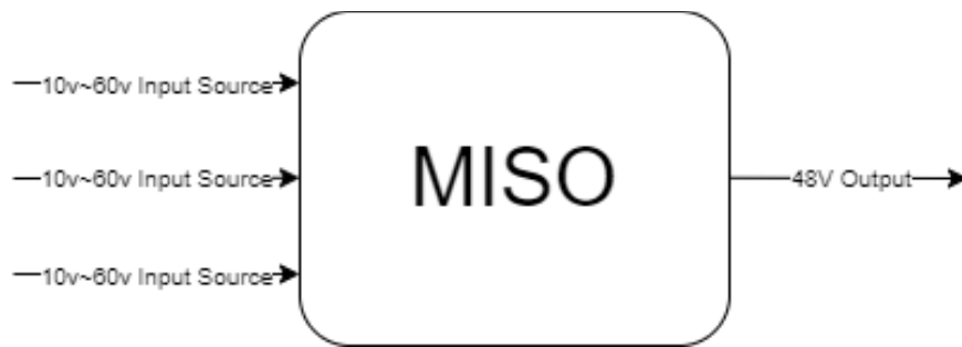
Figure 3.1: MISO Block Diagram Level 0
