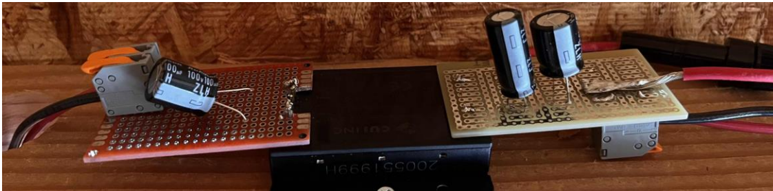
Figure 5.4 Wired DC to DC converter
