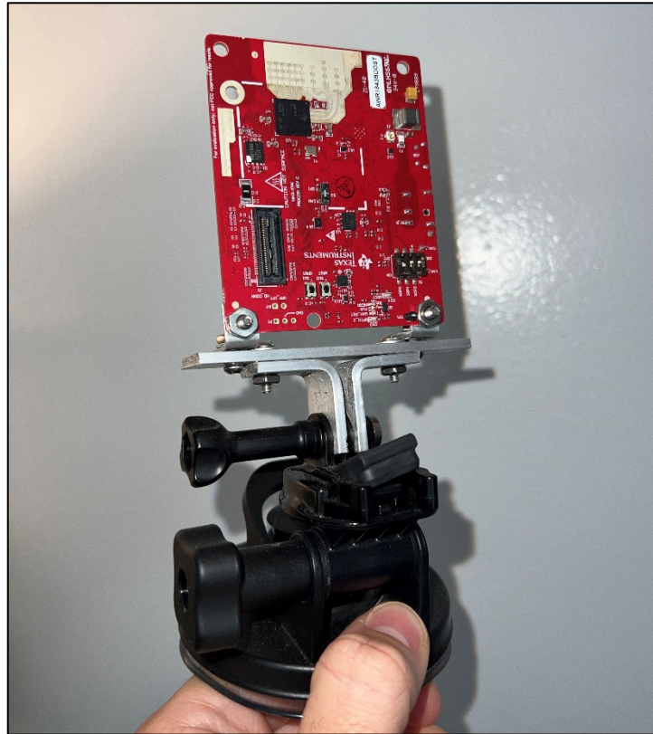
Figure 6.9 - Radar Mounting Setup
