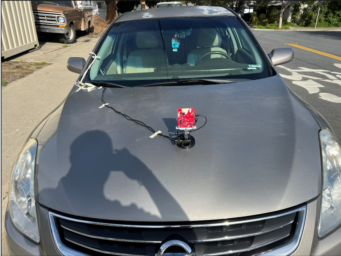
Figure 6.10 - Radar Mounted to Test Vehicle
