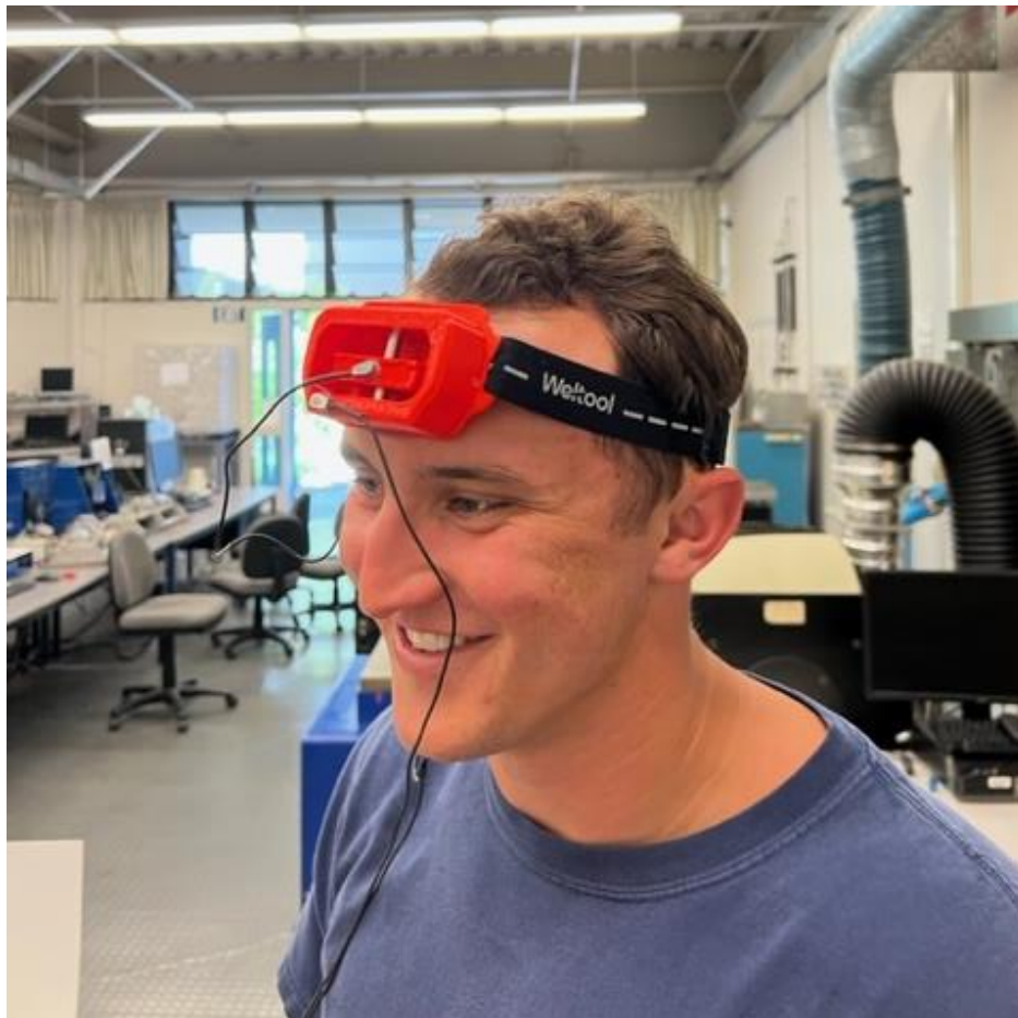
Figure 8 : Vibration Testing setup. Accelerometers attached to input and output locations of interest.
