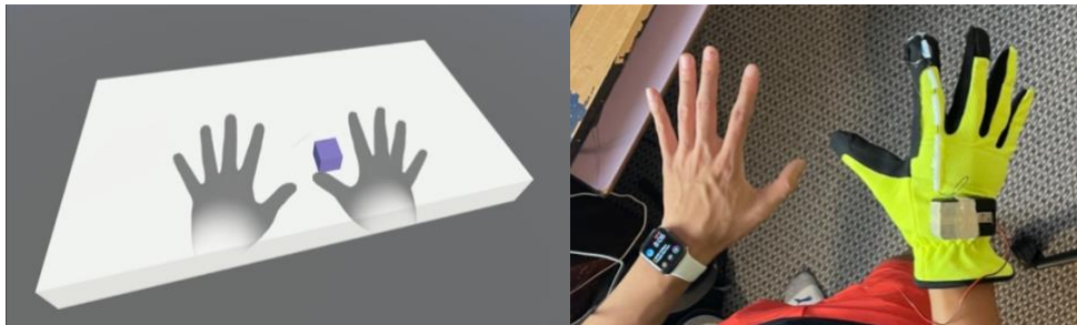
Figure 21. A screenshot of a playtest of the demo world showing hand tracking visualization, the white table, and the interactable cube. Side by side with the real world hand position.
