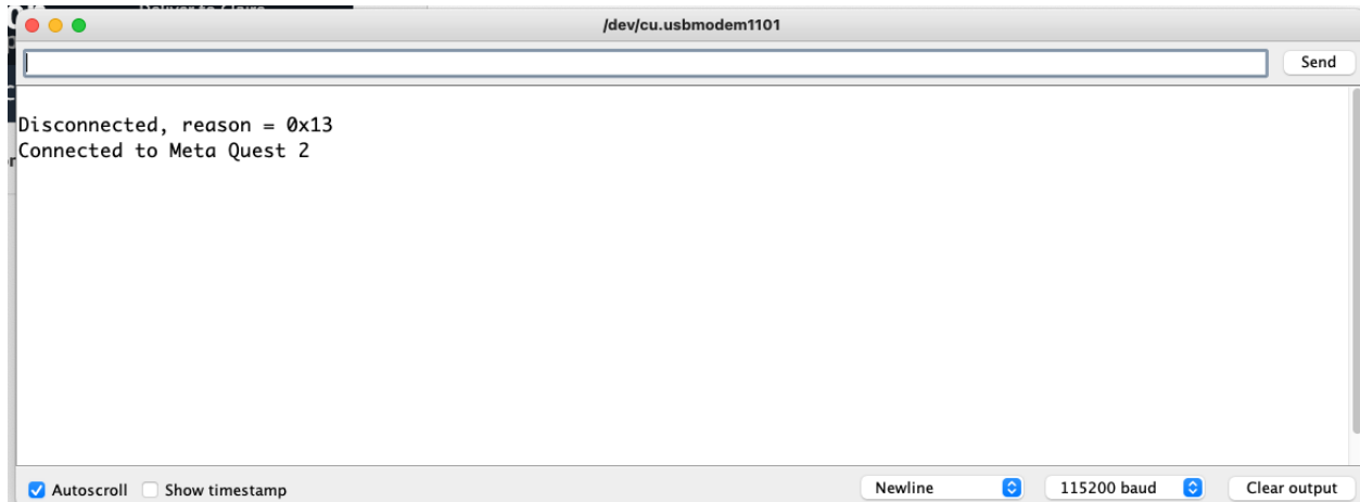
Figure 42. Arduino Serial terminal during connection to Meta Quest 2
