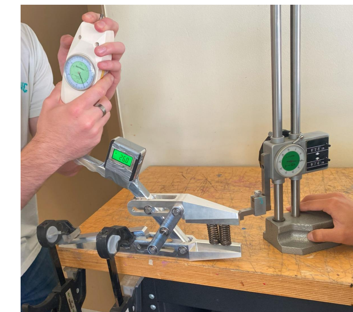
Mechanical Advantage using spring deflection
