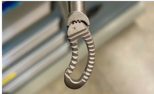
Figure 35. Orientation of spinal cage on inserter for spinal cage testing.
