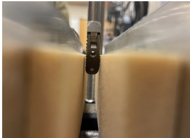
Figure 37. Spinal cage clamped between bone blocks in clamping fixture.
