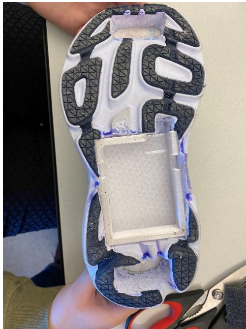
Figure 12: Final layout of shoe manufacturing with holes cut and case secured.
