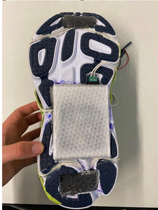
Figure 13: Final configuration of sensors, and wiring glued to sole of shoe.
