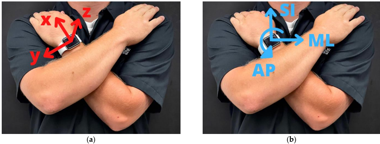
Figure 1. (a) Smartwatch's inertial coordinate system, showing the directions in which the smartwatch records acceleration, rotation rate, and gravitational field. (b) Global coordinate system, which contains the anterior-posterior (AP) direction, mediolateral direction (ML), and superior-inferior (SI) direction.
