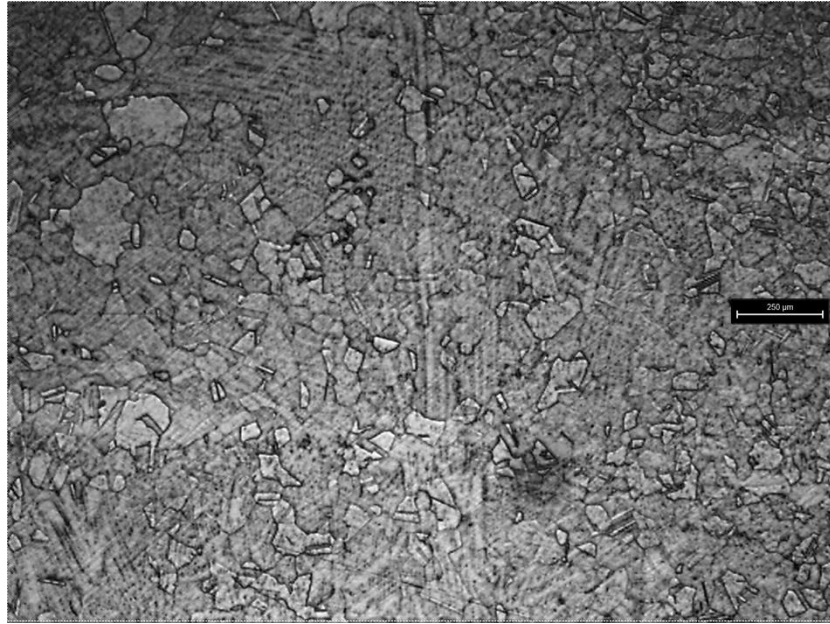
Figure 9: A microstructural image of the xz plane of a heat-treated DED Inconel 718 sample.
