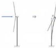
Figure 4.13: Illustration of a bottom-fixed wind turbine tower bending.
