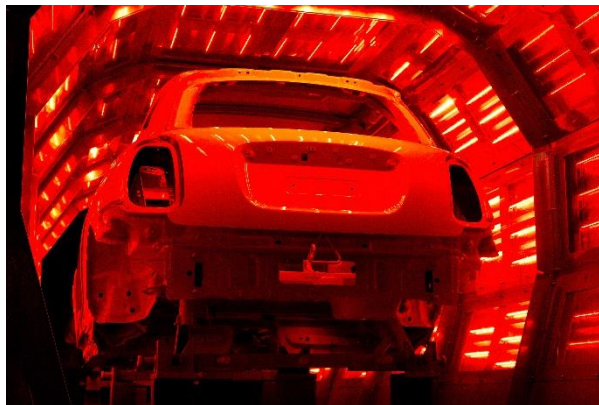
Figure 2.36: BMW MINI body-in-white being oven cured during one of the paint-baking steps [124].
