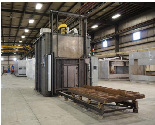
Figure 2.7: Example of a circulating air furnace used for industrial solution heat treatments of aluminium [78].
