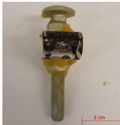
Figure 5.12: Water quenched and fast aged U-bend sample after 20 days of exposure to the salt spray fog environment.
