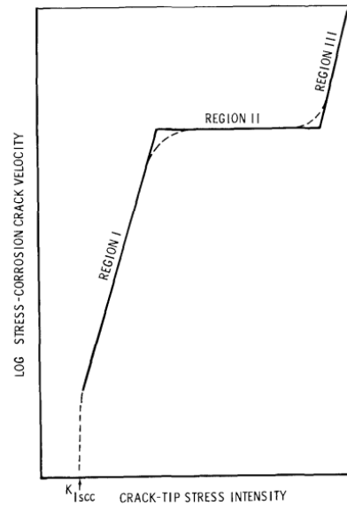
Figure 2.18: Schematic diagram showing the typical relationship between the stress intensity factor at the crack tip and the growth rate of the stress corrosion cracks for an aluminium alloy [97].
