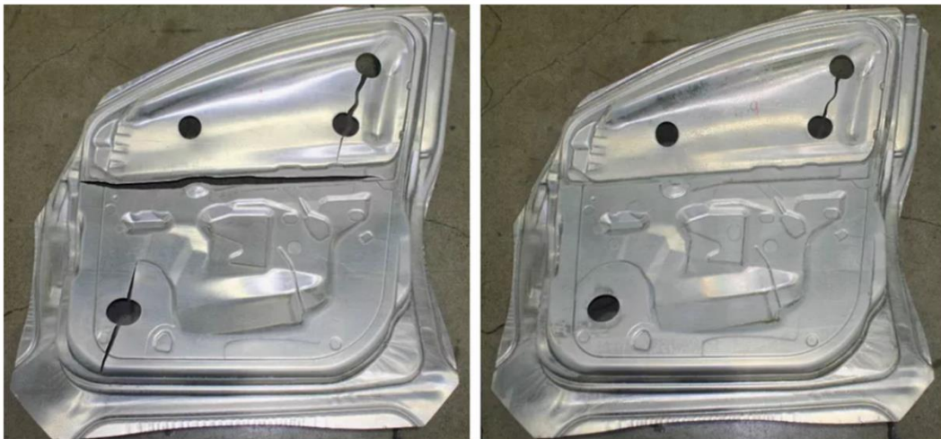
Figure 1.5: Aluminium auto panels formed at room temperature (left) and at 250°C (right) [20].
