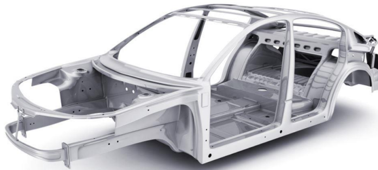
Figure 1.1: An example of a car body with a monocoque design [1].
