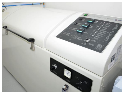
Figure 3.27: Liebisch Constamaticwin SK 400 M-TR salt-spray chamber.
