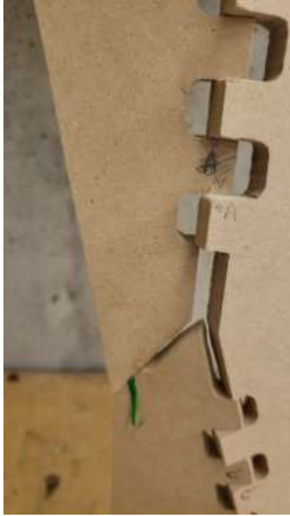
Figure 82 Edges Finger Not Fit Accordingly
