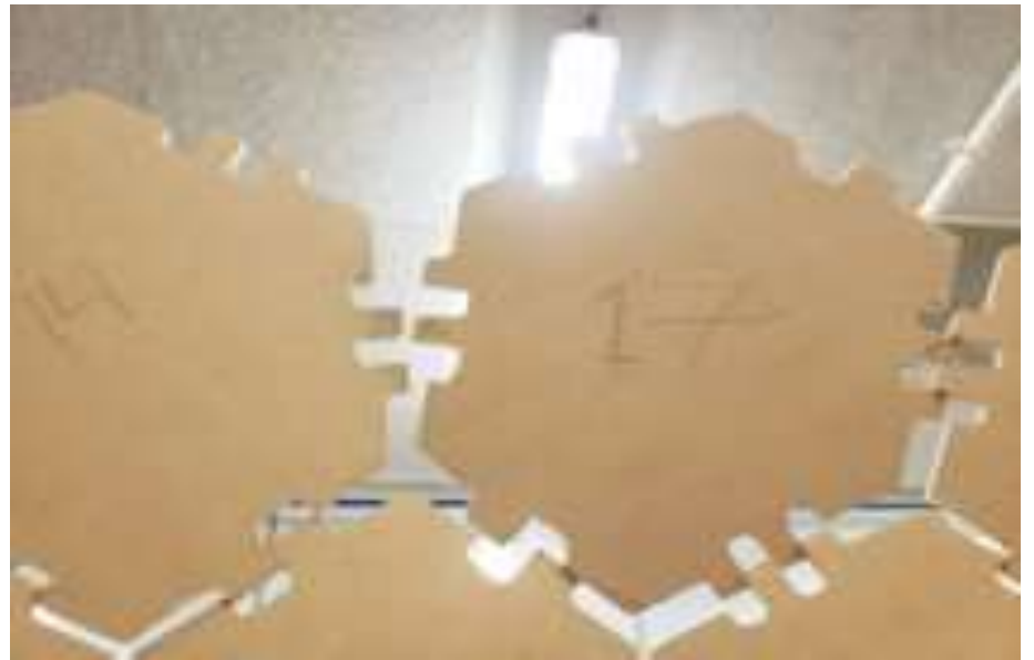
Figure 85 Center Gap in Segmental Problem
