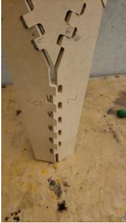
Figure 81 Gap between Segments
