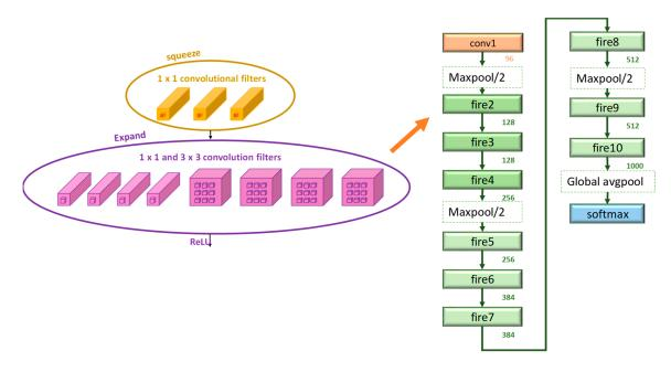
Figure 6. SqueezeNet architecture.
