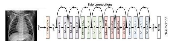
Figure 4. Structure of ResNet18.
