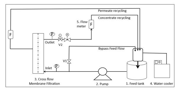
Figure 1. Crossflow filtration setup used for the pure water permeability and scaling tests [8,14].
