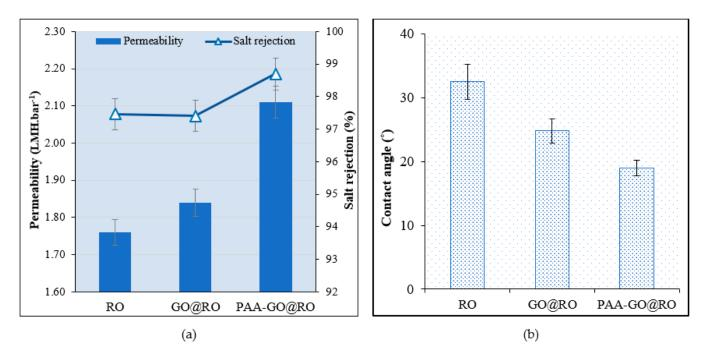
**Figure 7.** Results of (**a**) Membrane pure water permeability and salt rejection, (**b**) Water contact angle of the bared and optimized modified membrane.
