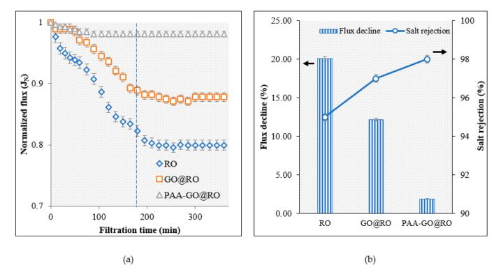
**Figure 11.** Inorganic fouling tests for the membranes (**a**) Decline of normalized flux with time, (**b**) Comparison of flux decline and salt rejection at the end of experiments.
