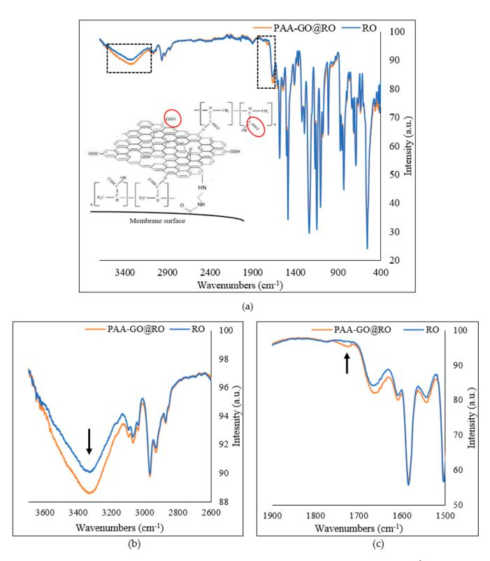
**Figure 9.** ATR-FTIR spectra of the membranes (**a**) complete spectra  $3900-400 \text{ cm}^{-1}$ ; (**b**) spectral range  $3900-2900 \text{ cm}^{-1}$ ; (**c**) spectral range  $1900-1500 \text{ cm}^{-1}$ .
