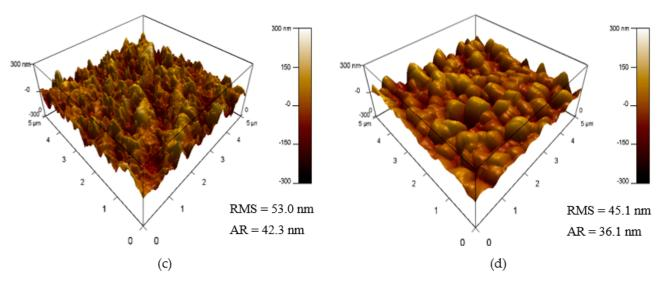
**Figure 8.** SEM micrographs and AFM images of the membranes (**a**,**c**) RO membrane; (**b**,**d**) PAA-GO@RO optimized membrane.
