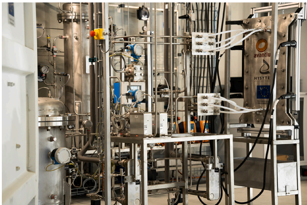
Fig. 11. Pre-pilot plant unit for formate production [201].
