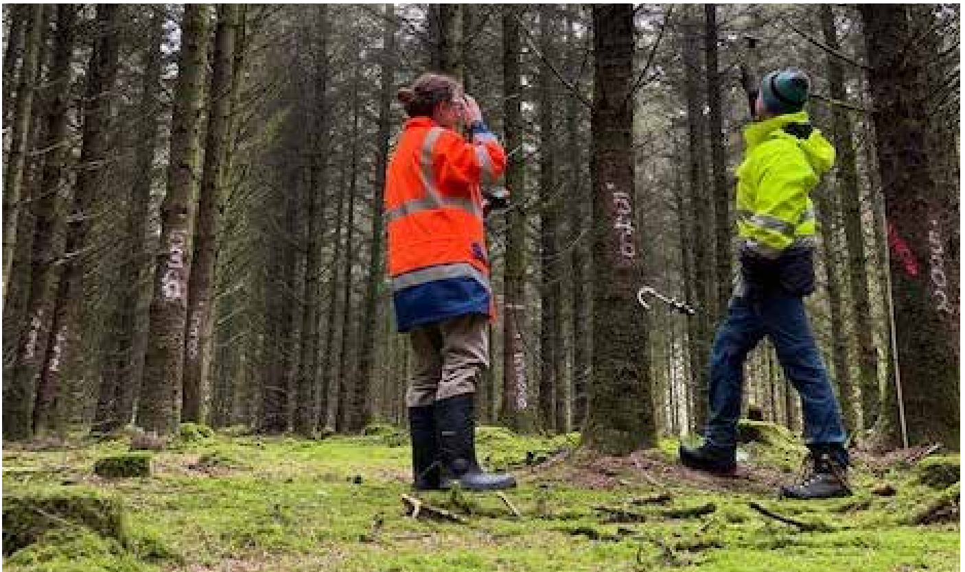
Grace Jones (Postdoctoral researcher, Teagasc) and Mark Whelan Spain (Bachelors Forestry student, UCD) measuring Time-of-Flight with the TreeSonic timer (Fakopp, Hungary) at Fossy Hill
