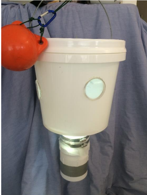
Figure 1. Image of light trap made from a three-gallon bucket and inverted funnels.
