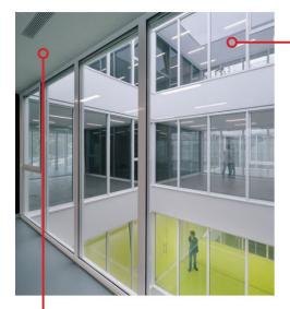
Central open courtyard allow max natural daylighting into the entire building as the floor layout are wrapped around the courtyard.
