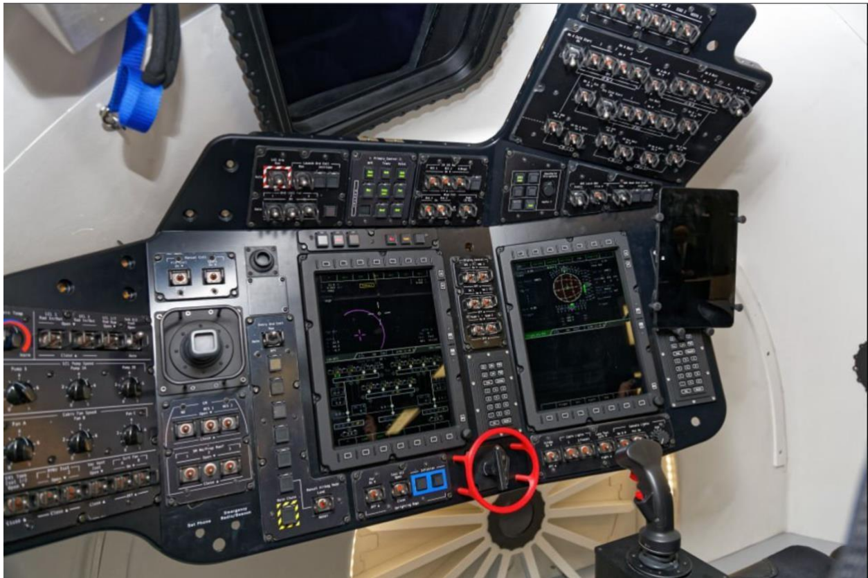
Figure 26: Boeing Display of Starliner Cockpit that a pilot would control during mission profiles [21]
