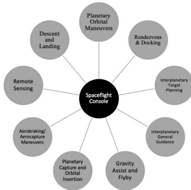
Figure 34: Diagram showing the top-level functions of proposed Spaceflight Console
