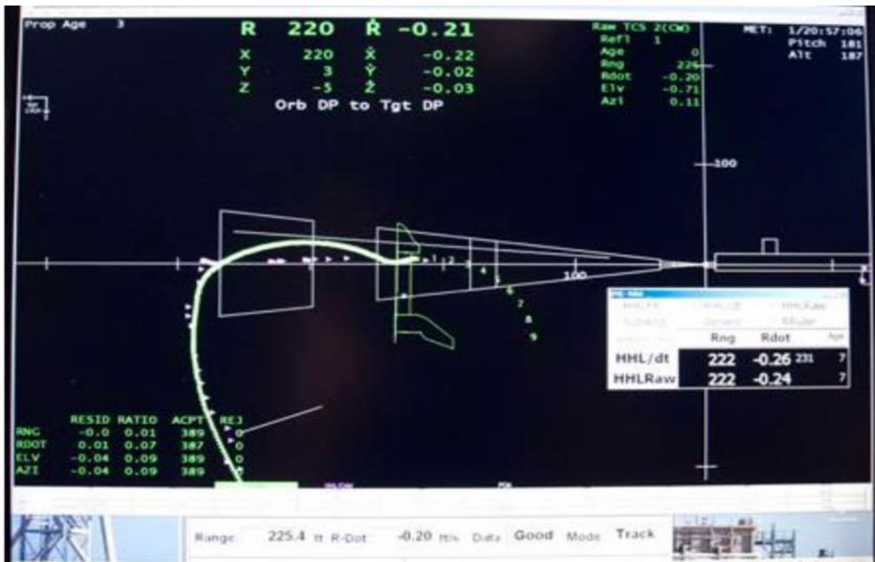
Figure 1: RPOP onboard laptop display showing relative position data and providing 2D visualization of the Space Shuttle's approach to docking with ISS [33]
