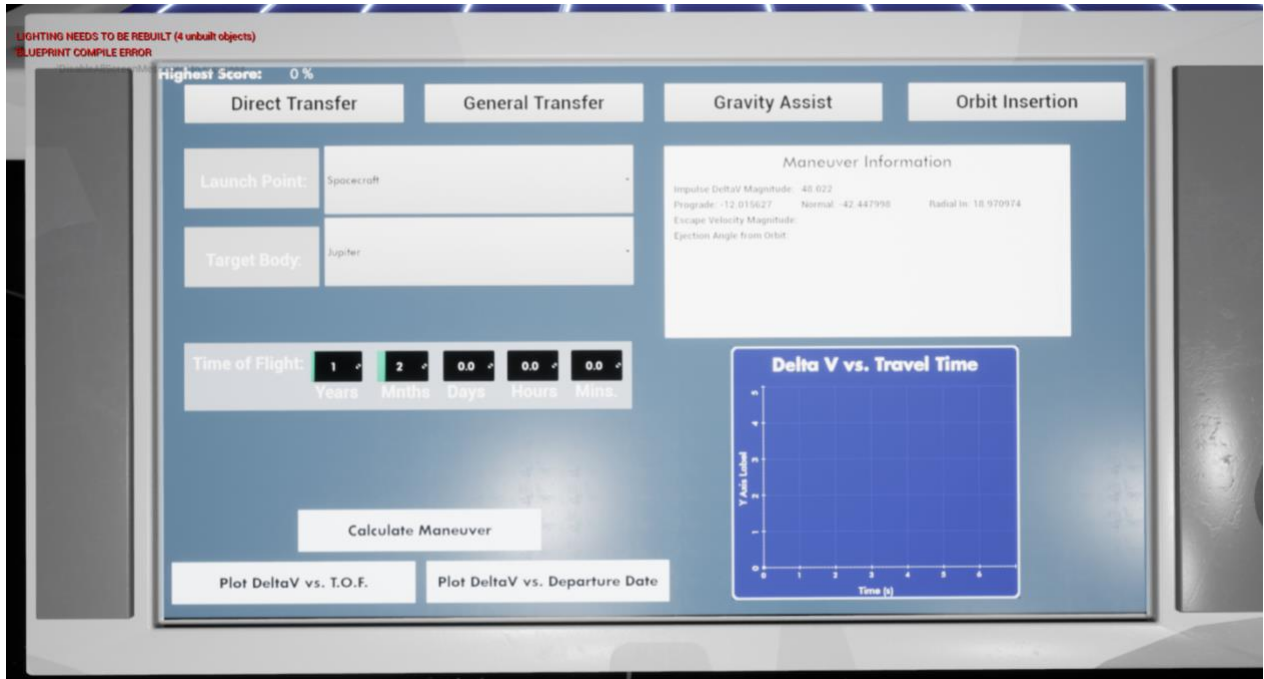
Figure 49: Spaceflight Console from Pilot Perspective for Lambert Target from Spacecraft to Jupiter
