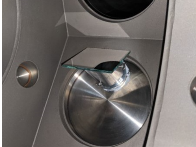
Figure 3.24: Diagnostic Station #1 retro-reflecting mirror positioned on a 45° octagonal face. The custom mirror mount has a main cylindrical body, which is adhered to the vacuum flange via vacuum-compatible epoxy, and an outer cylindrical housing with a 45° section milled out of the cylinder such that mirror remains horizontal when installed. The mirror is also adhered to the mount with vacuum-compatible epoxy. The two cylindrical bodies allow a rotation that can help adjust the back-reflection. Set-screws are used to lock in the rotation position.
