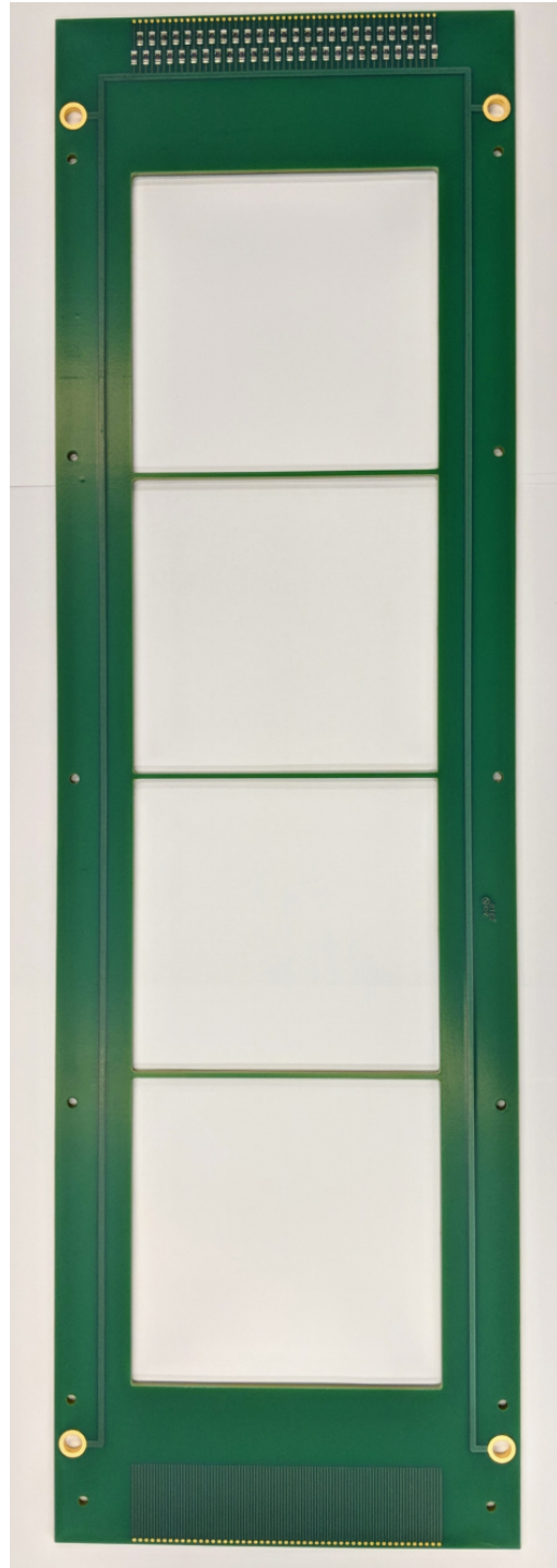
Figure 6: Back view of the bare Y-plane cathode of the PPAC detector before connecting the Be-Cu wires
