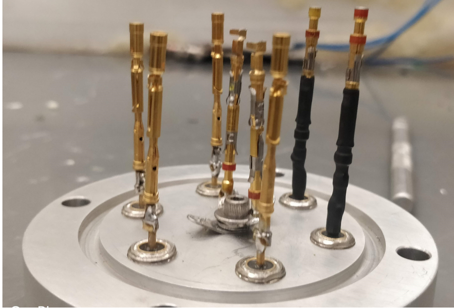
Figure 14: Connector used to connect the internal wires to the external electronics
