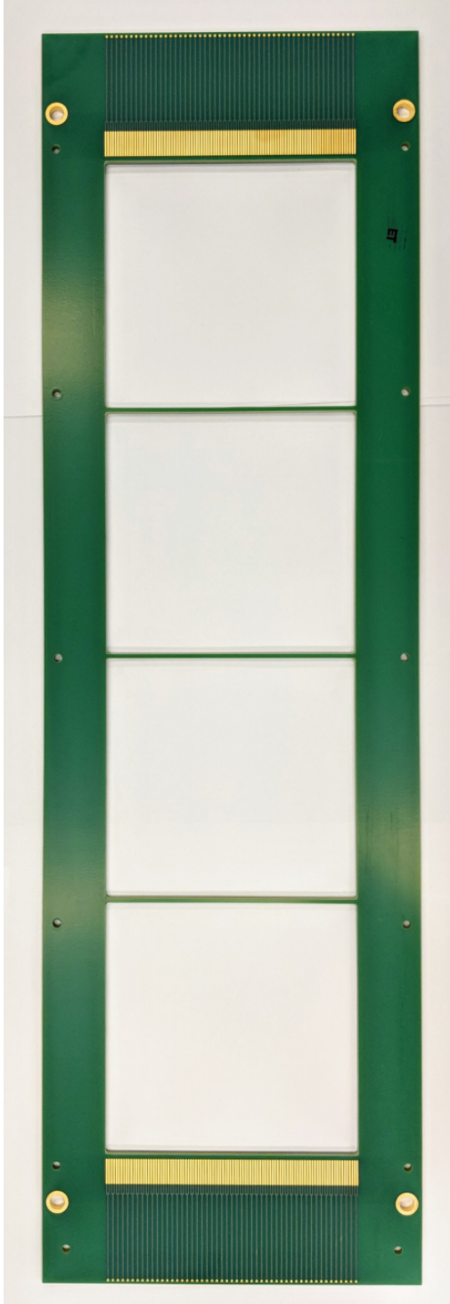
Figure 5: Front view of the bare Y-plane cathode of the PPAC detector before connecting the Be-Cu wires
