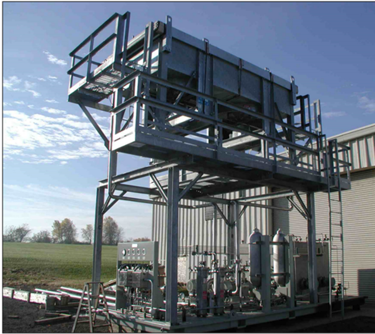
Figure 8: Air Heat Exchanger Mounted on the Lube Oil System (Image courtesy of G.J. Oliver, Inc.)
