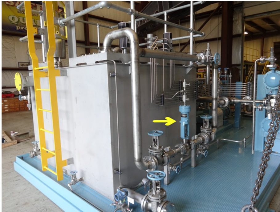
Figure 2: Positive Displacement Pump Back-pressure Control Valve (Image courtesy of G.J. Oliver, Inc.)
