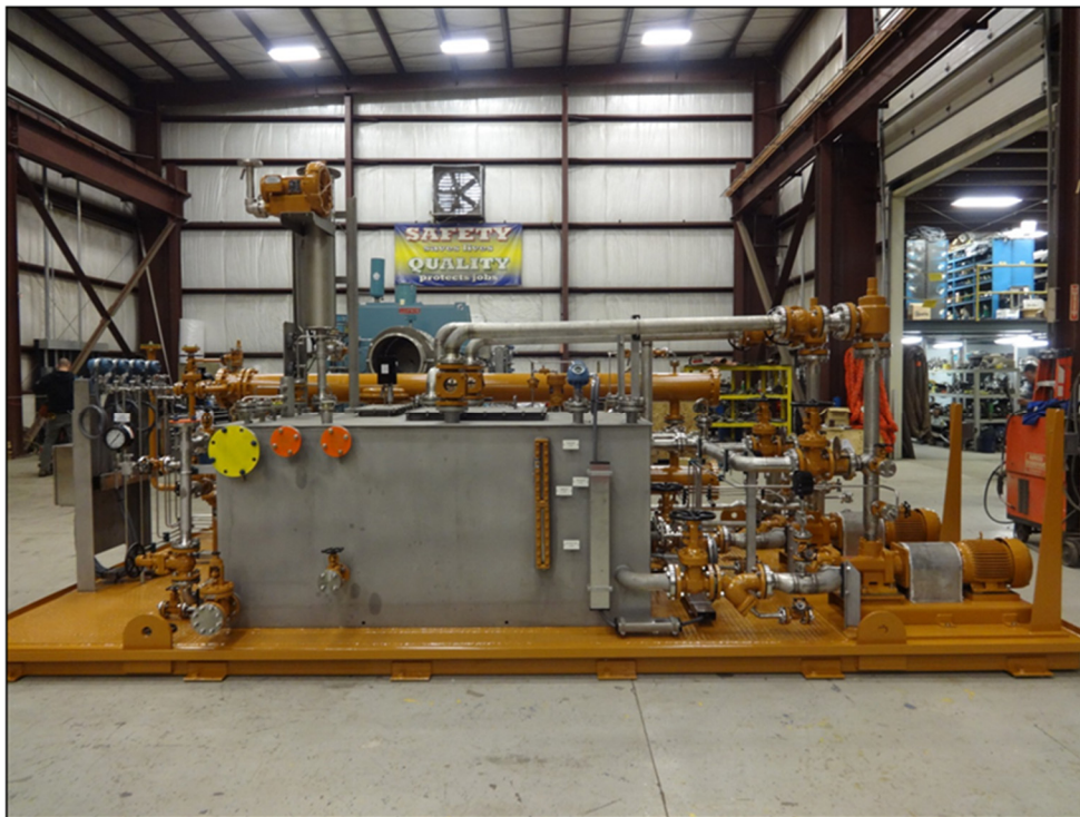
Figure 25: Typical Special Purpose Lube Oil Console (Image courtesy of G.J. Oliver, Inc.)
