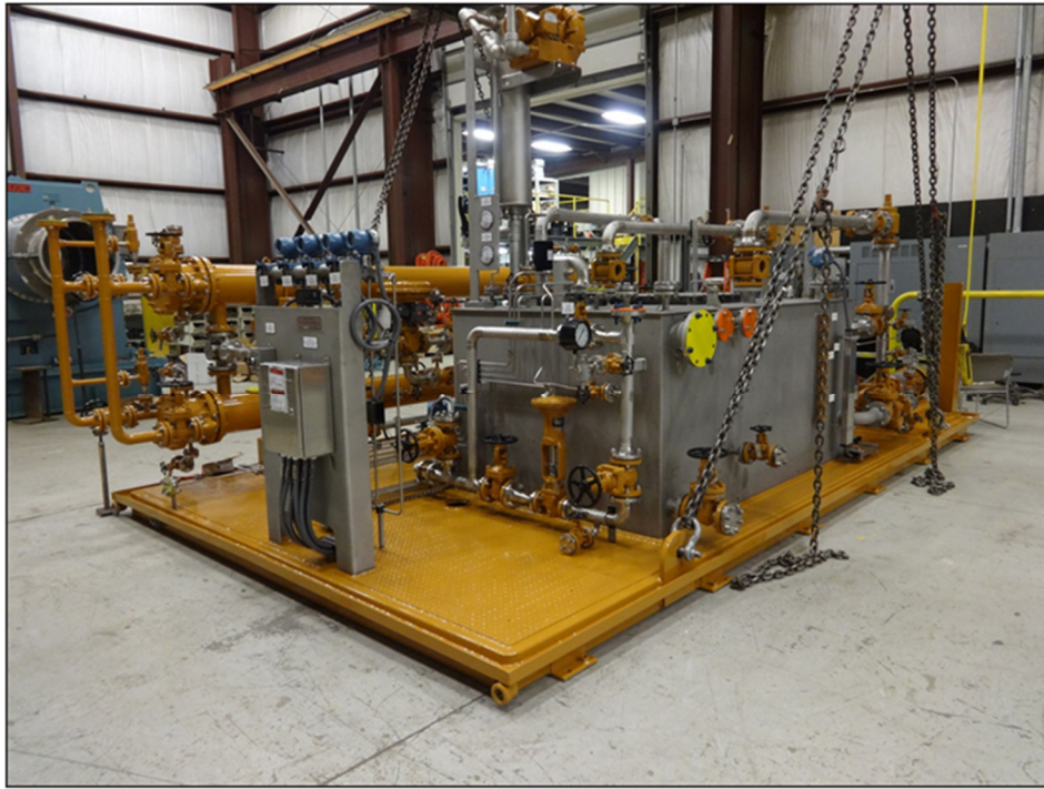
Figure 26: Typical Special Purpose Lube Oil Console (Image courtesy of G.J. Oliver, Inc.)
