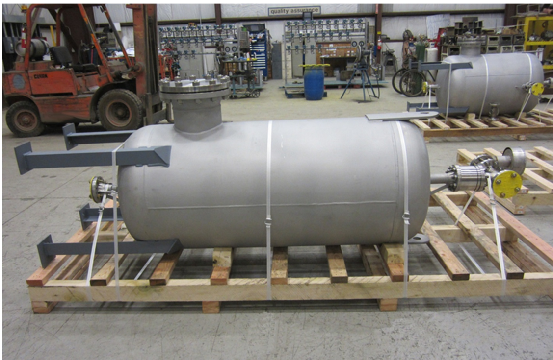
Figure 31: Vertical Pressurized Lube Oil Rundown Tank (Image courtesy of G.J. Oliver, Inc.)
