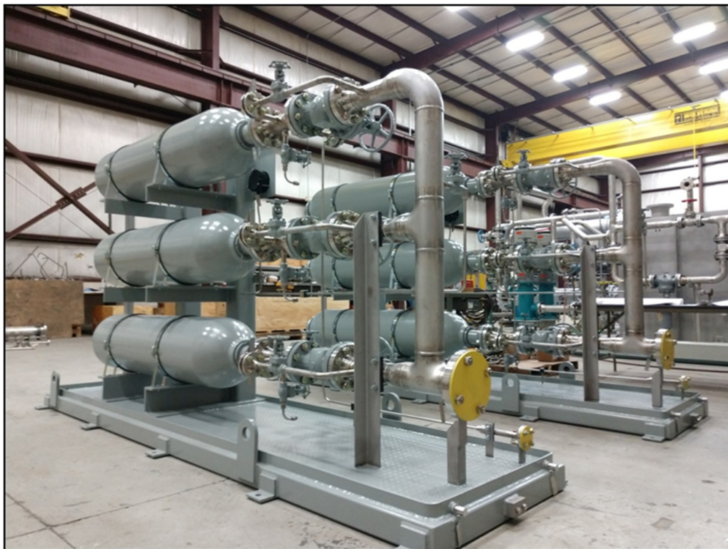
Figure 20: Multiple Parallel Horizontal Accumulators (Image courtesy of G.J. Oliver, Inc.)
