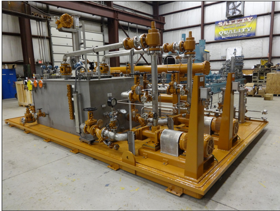
Figure 24: Typical Special Purpose Lube Oil Console (Image courtesy of G.J. Oliver, Inc.)
