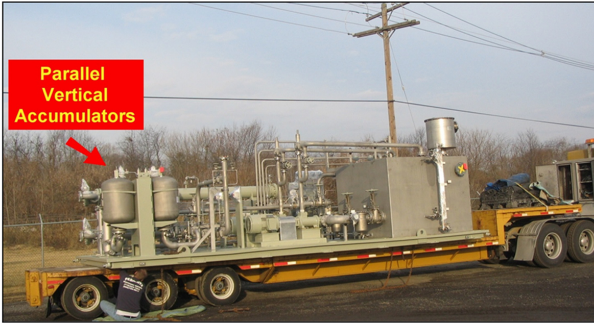
Figure 21: Multiple Parallel Vertical Accumulators (Image courtesy of G.J. Oliver, Inc.)
