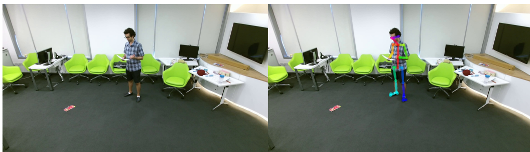
Figure 4.3: The original frame(left) and the frame with skeleton(right) for a false positive case of Skeleton based models 2
