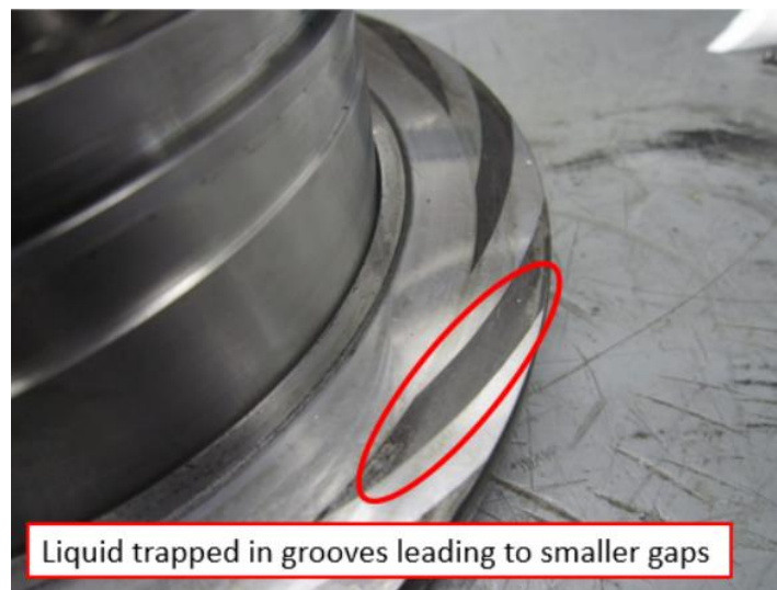
Figure 22. Grooves Filled with Liquid
