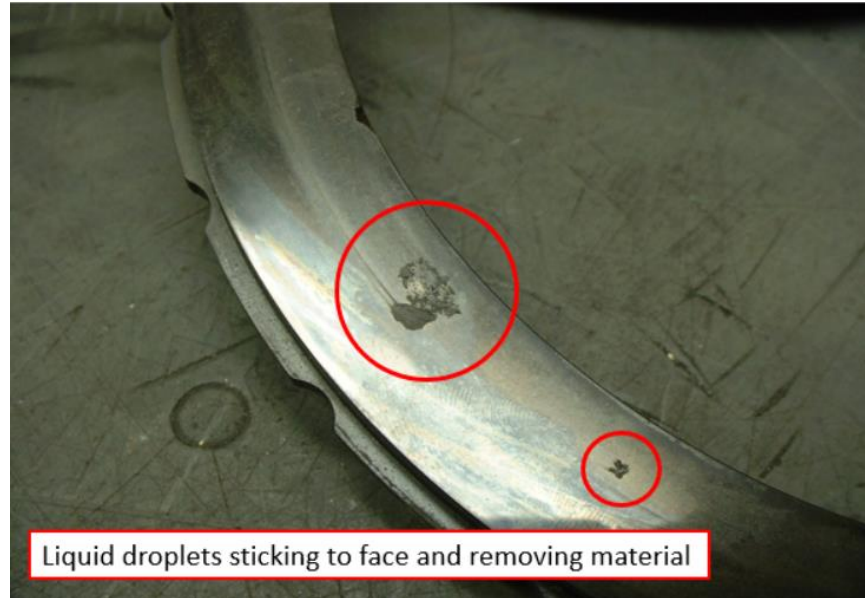
Figure 21. Liquid Build Up in a Seal
