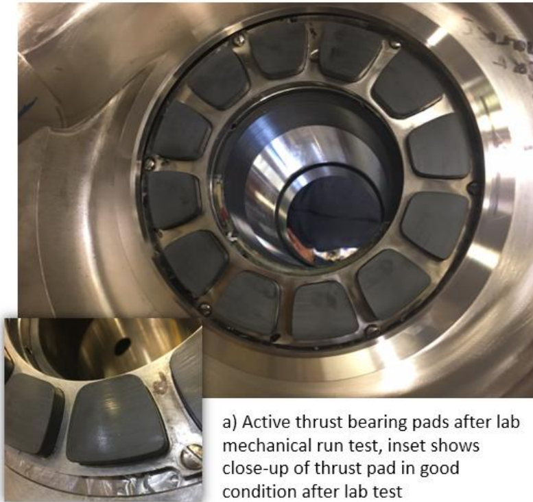
Figure 39: Thrust and journal bearings are in good condition post mechanical run test after bearing rub issue was fixed
