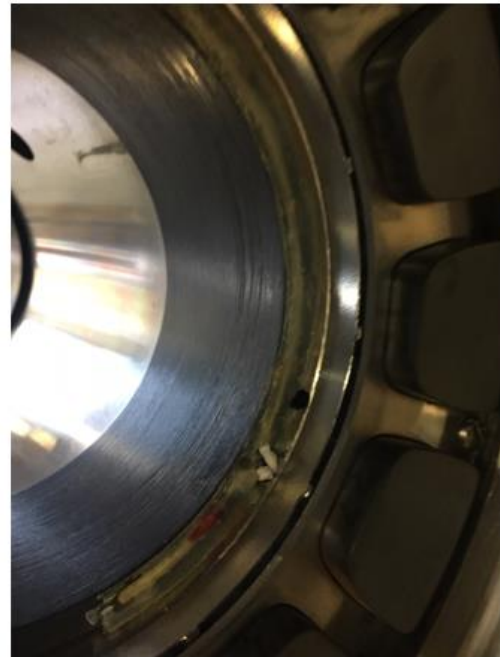
b) Journal bearing in good condition after lab mechanical run test
