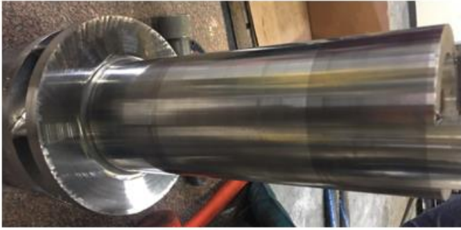
a) Turbine back shroud (running face for active thrust bearing) & shaft surface in good condition after lab test
