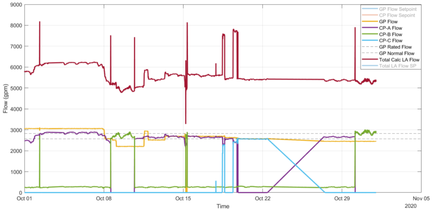
Figure 42: Operational data of turbocharger and circulation pump lean amine flow rates of HSBH Unit 1 AGR plant for Oct 2020
