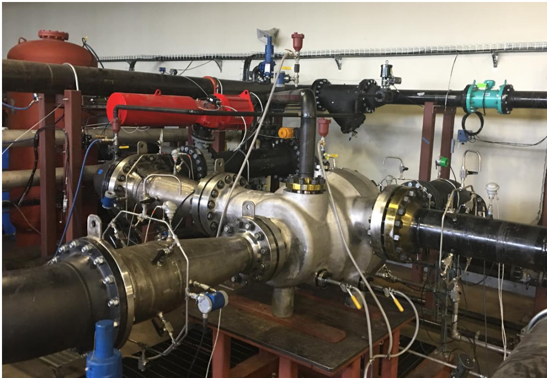
Figure 31: Turbocharger FAT setup showing instrumentation at inlets and outlets of the turbocharger
