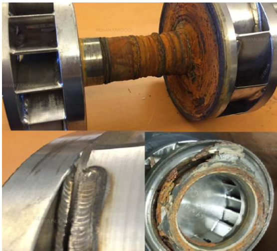
Figure 6: Experience of catastrophic damage history of hydraulic turbocharger on water service
