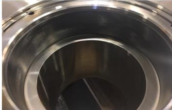
c) Pump wear ring in good condition after lab test
