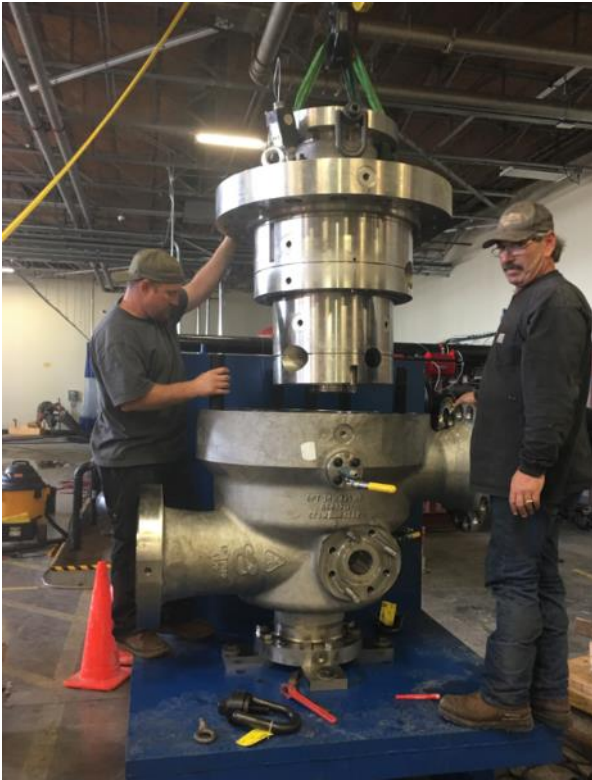
Figure 13: Installation of cartridge in turbocharger casing for FAT
