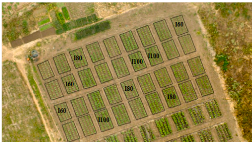
Fig. 2. Experimental plot with irrigation application at 100% (I100), 80% (I80) and 60% (I60) of calculated crop water requirements.
