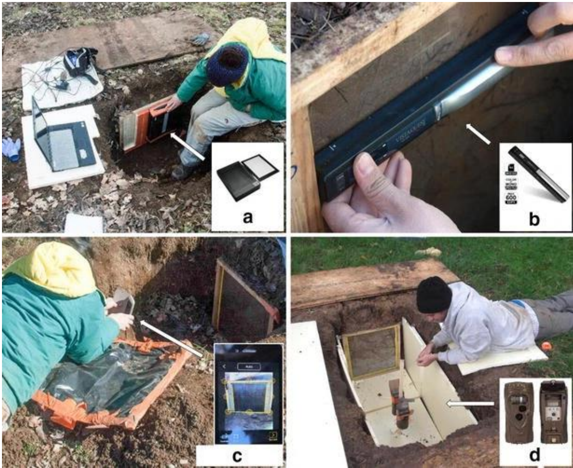
Figure 2.4 An example of a small rhizotron installation. Mohamed et al compared the efficacy of 4 different image acquisition platforms in rhizotrons. a , flatbed scanner, b handheld scanner, c smartphone scanner, d time lapse camera. Figure is from Mohamed et al. and used under CC-BY 4.0 License [72].
