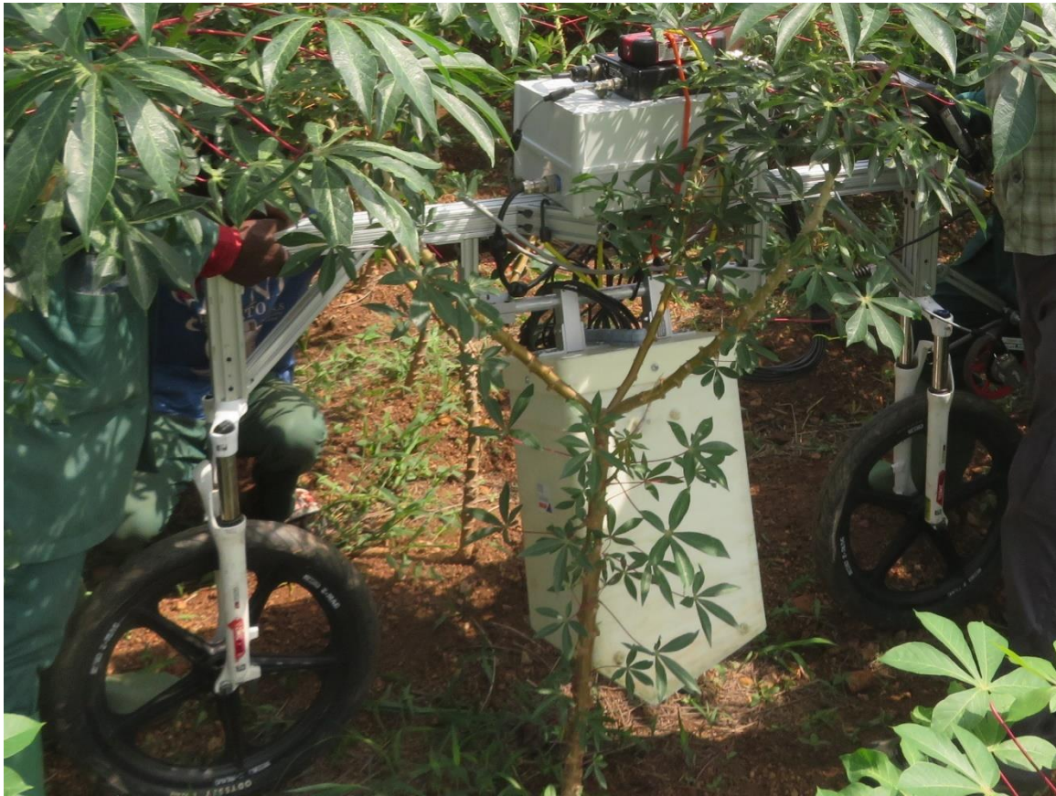
Figure 5.1 The GPR cart traveled on 2 wheels to accommodate the narrow row spacing, but still required some branches be pulled back to allow passage. The electronics were mounted on top, the tablet computer at the rear, and the antenna slung beneath at an angle towards the plant row.
