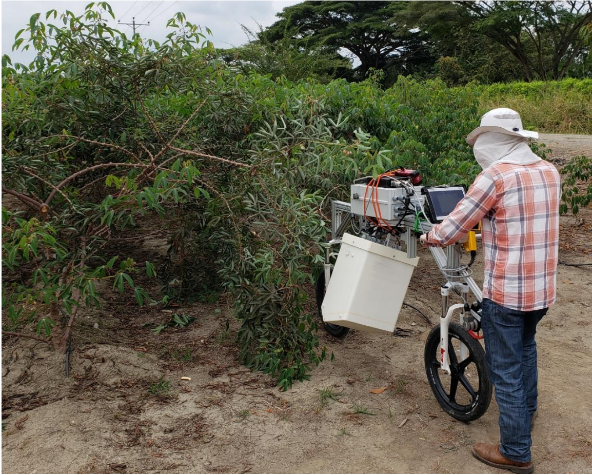
Figure 4.3 The GPR cart ran on two wheels and carried the antenna array approximately 35 cm above the ground, allowing the array to be angled towards the center of the plant. The bicycle-like configuration allowed the cart access between plant rows. Some branches required lifting to allow passage.
