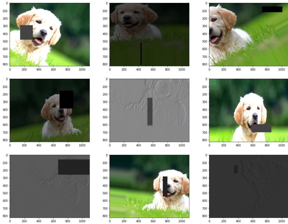
Figure 3.5: Examples of images generated with combination of all eight augmentation types. Flip and sobel filter was randomly applied to images with probability of 0.5.
