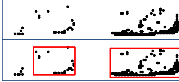
Figure 2.12: DSBSCAN Clustering on a undilated BeV LiDAR image with two vehicles. The left cluster is undesirable due to the sparsity of the data and under-clustering.
