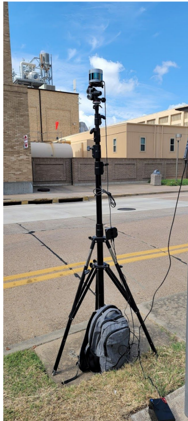
Figure 3.1: Experimental Setup for TAMU_03. A VLP-32c is mounted on a heavy-duty tripod, and connected to a 12v battery source. Ethernet is connected from the LiDAR to a laptop for data collection
