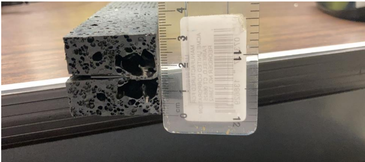
Figure 116. Detailed View of Damaged Area of Sample B4_1
