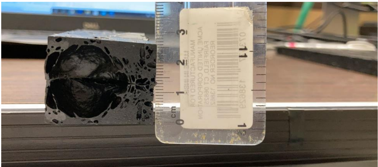
Figure 64. Detailed View of Damaged Area of Sample A3_2
