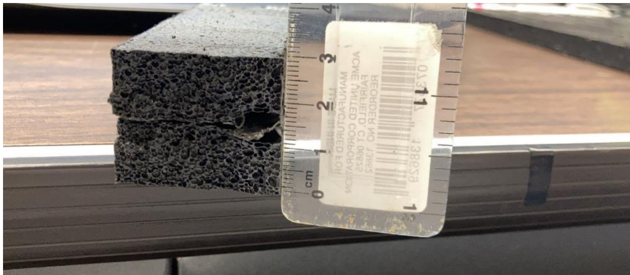
Figure 74. Detailed View of Damaged Area of Sample B3_2
