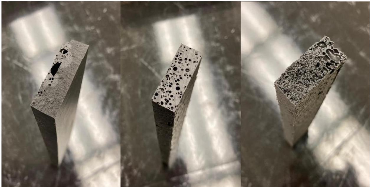
Figure 31. Samples with 8%, 30% and 50% V_{VF}
