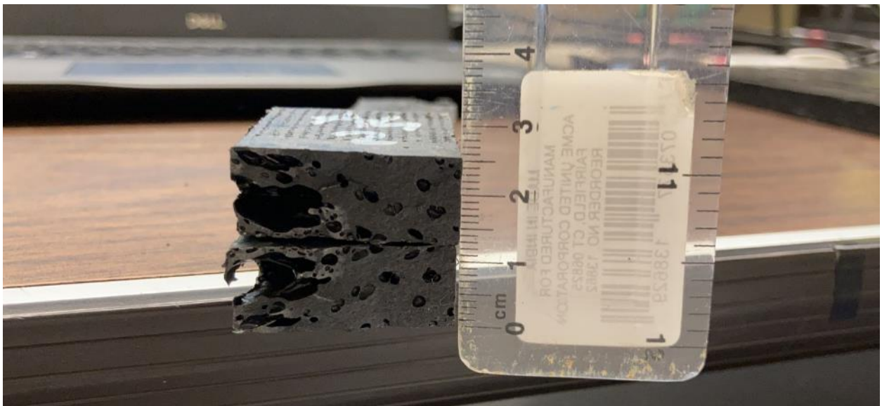
Figure 66. Detailed View of Damaged Area of Sample A4_2
