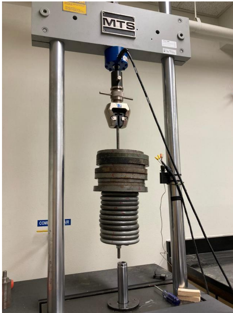
Figure 26. Calibration of the Load Cell
