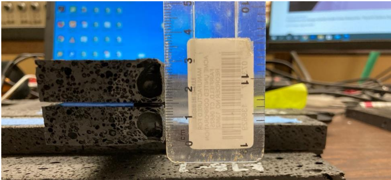
Figure 50. Detailed View of Damaged Area of Sample B4
