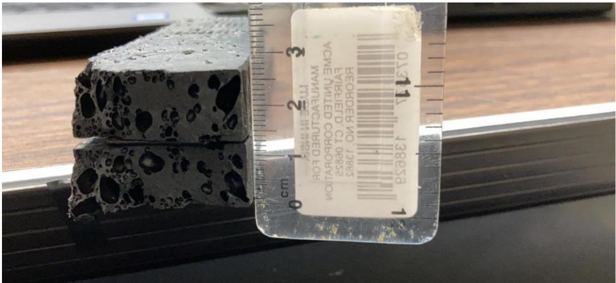
Figure 128. Detailed View of Damaged Area of Sample D5_1
