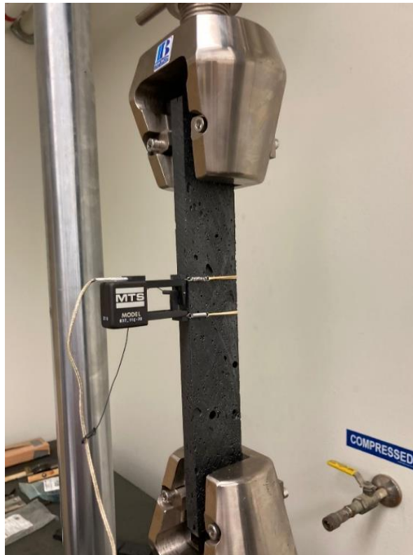
Figure 29. HDPE Composite Sample Mounted for Testing
