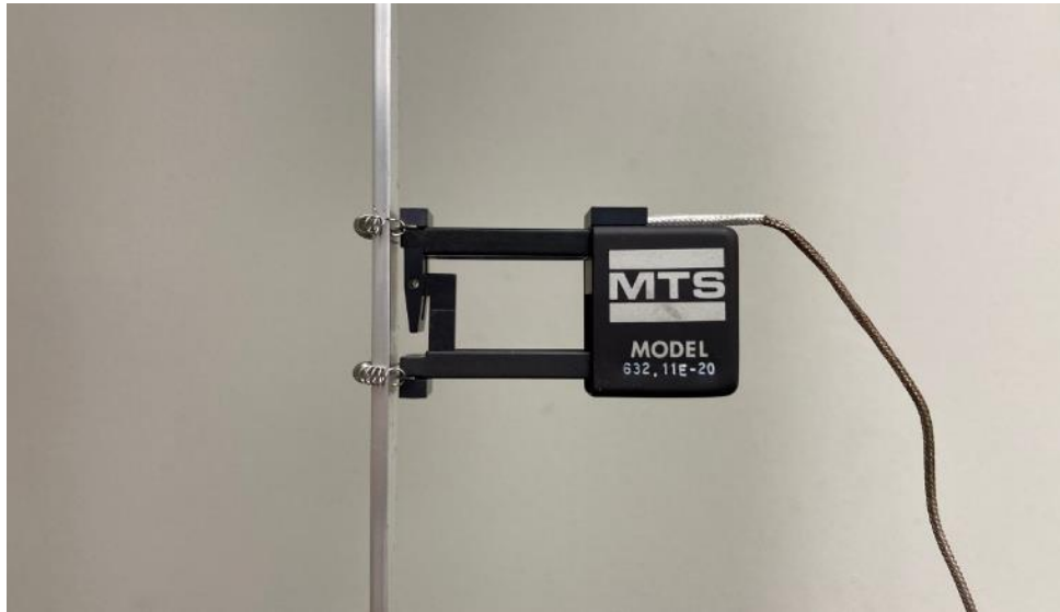
Figure 27. Extensometer Calibration During the Aluminum 6061 Test
