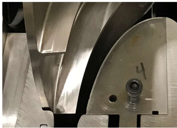
Figure 11 Unshrouded impeller with contour ring ( rotor & contour ring not in final running position )
