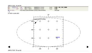
Shaft centerline plots indicated no change in shaft position
