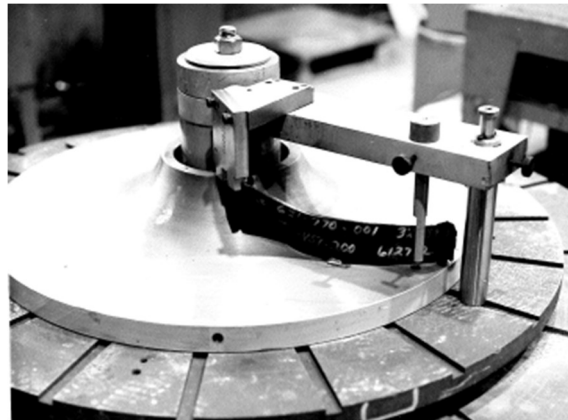
Figure 15 – Locator positioning formed blade on hub for welding
