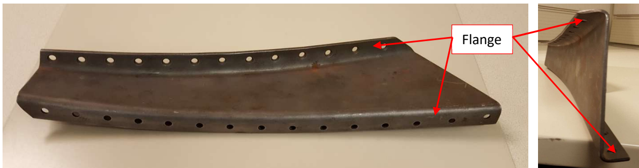
Figure 10 – “Z” blade – note flanges in photo at left and “Z” shape in photo to the right
