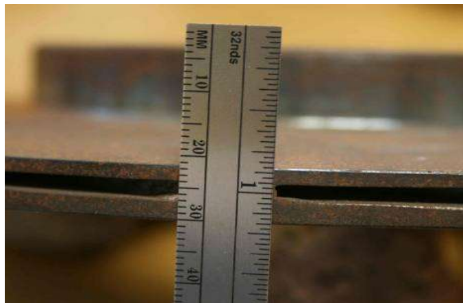
Figure 21 – Impeller with very narrow blade height – 0.11” (2.8mm)
