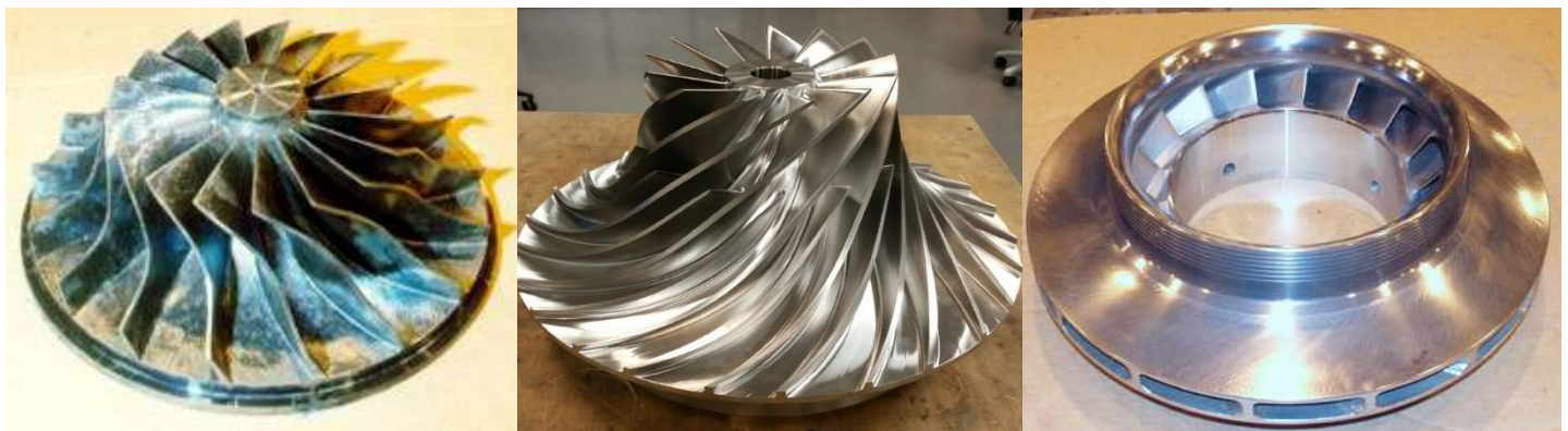
Figure 9 – Impeller Types – Unshrouded at left and center – Shrouded at right
