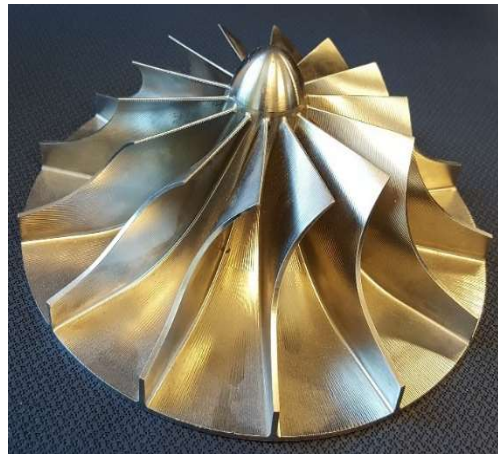
Figure 16 – 5-axis milled open impeller
