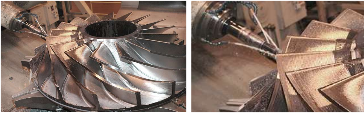
Figure 19 – Point milling blades integral with hub – See milling ridges / serrations at
