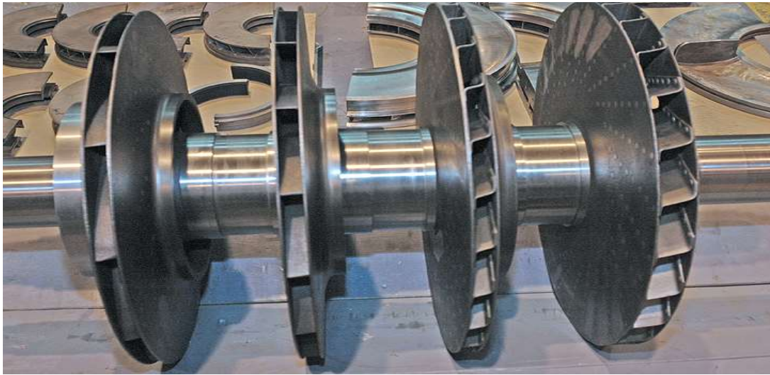
Figure 11 – Rotor with riveted impellers (“through blade” to left and “Z” blade to right)
