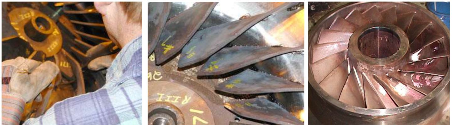
Figure 17 – Various steps in three-piece welded impeller assembly.
