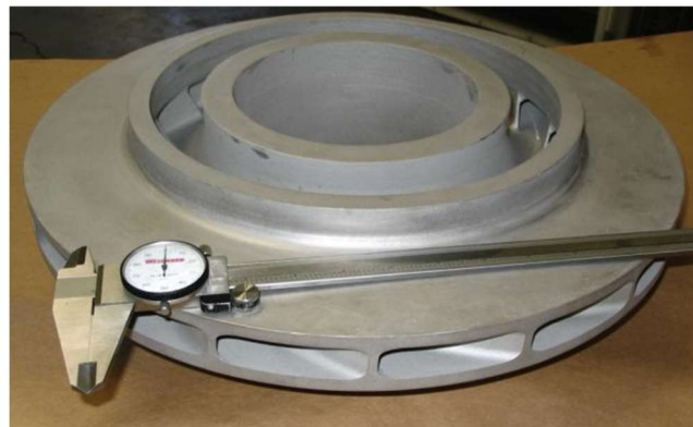
Figure 29 – An impeller built from powdered metal
