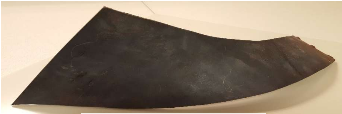
Figure 14 – Impeller blade formed from plate
