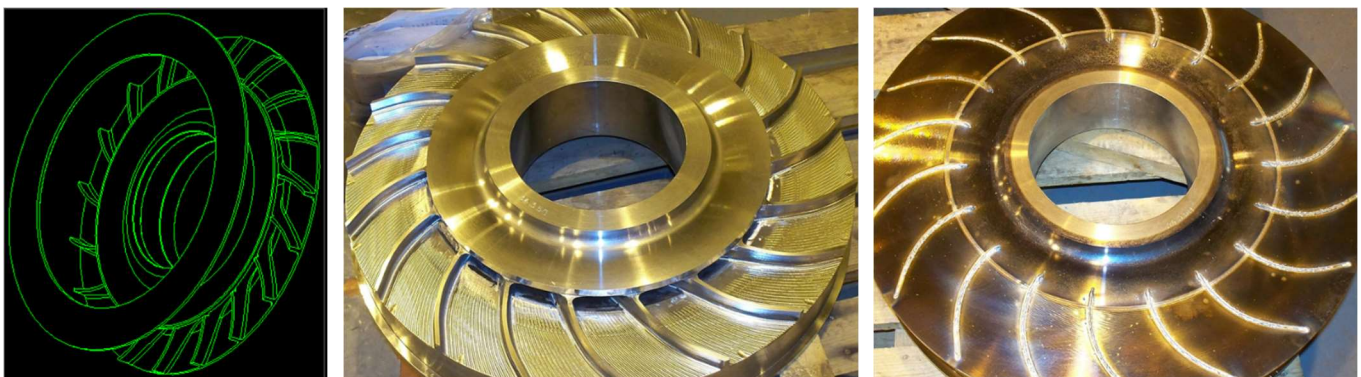
Figure 26 – Graphic rendition of cover plate and single piece section at left – Single piece machined section in center -- Photo of impeller with cover plate EB-welded in place at right
