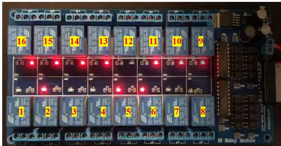
Figure 3.4: Relay Output for Hexadecimal Payload of F732
