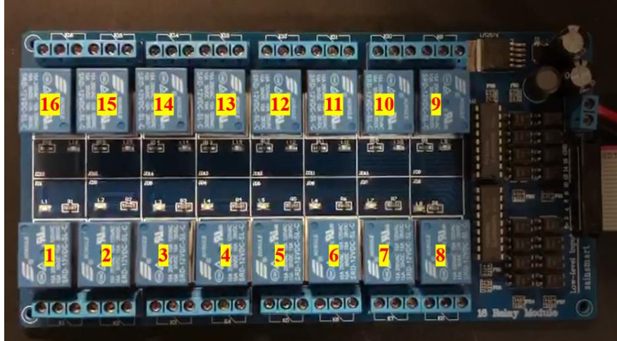
Figure 3.2: Relay Output for a Hexadecimal Payload of 0000
