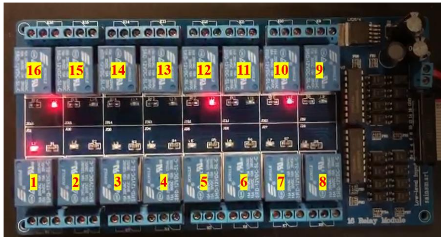
Figure 3.1: Relay Output for a Hexadecimal Payload of 8A01
