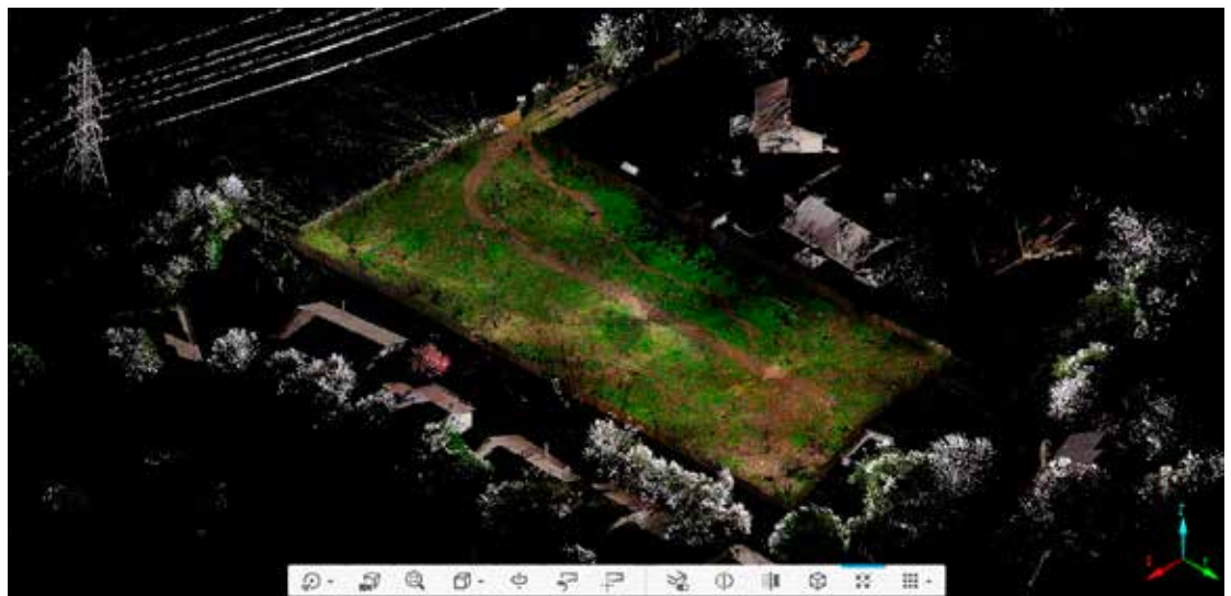
Figure 8: Isometric view (from West looking East]. Screenshot of color point cloud from FARO Scene: trees digitally cropped.
