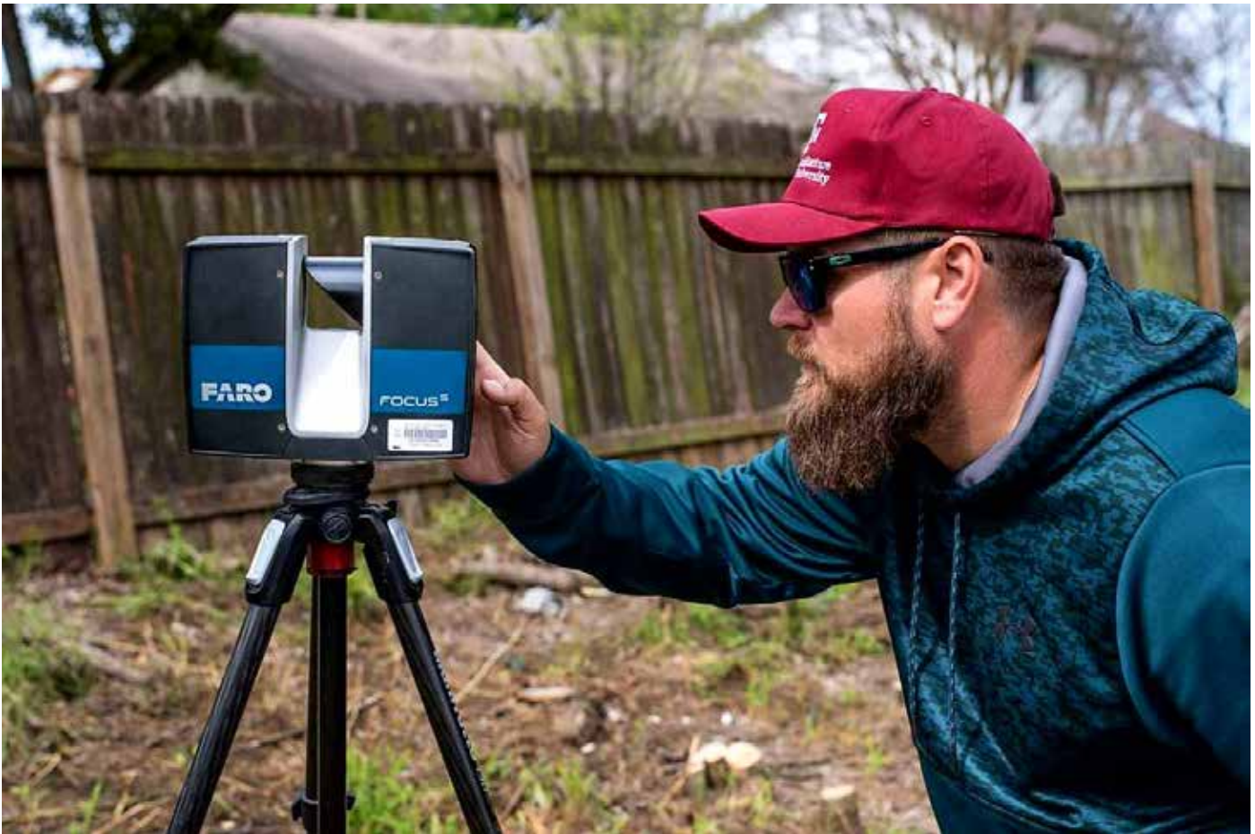
Figure 3 (above). Graduate student Andrew Bilingsley operating the FARO Focus s350 laser scanner.
