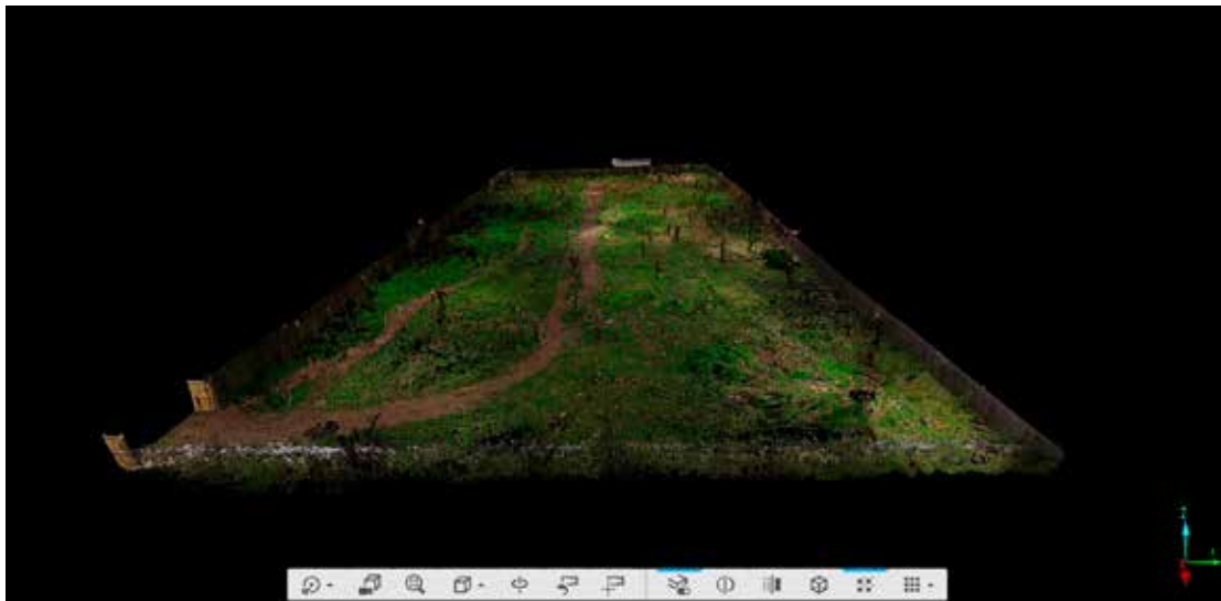
Figure 10: Perspective view (from Northeast looking Southwest). Screenshot of color point cloud from FARO Scene: trees and surrounding houses digitally cropped.
