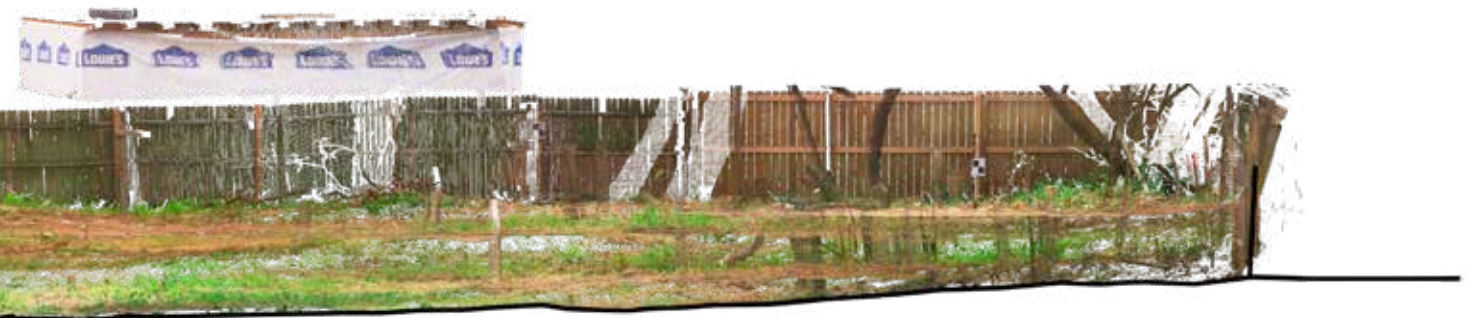
Figure 16. Transverse Section (Southeast-Northwest Axis, looking Southwest). Orthophoto of point cloud export from FARO Scene.
