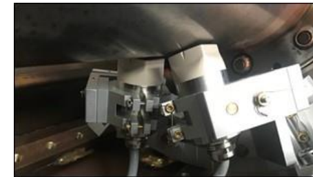
Torsional Vibration Sensors Installed at LS Coupling (HS Similar)
