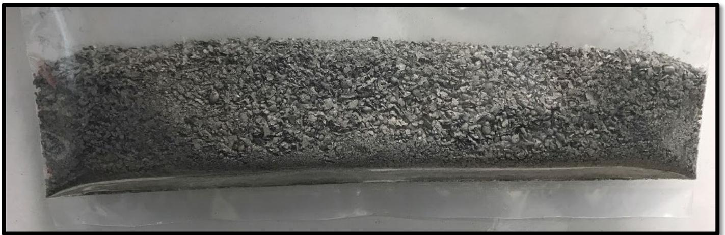
*Figure 5. Photo of Ring Magnet in Pieces (in a plastic bag) After Testing in a Pressurized Hydrogen Gas Environment*
