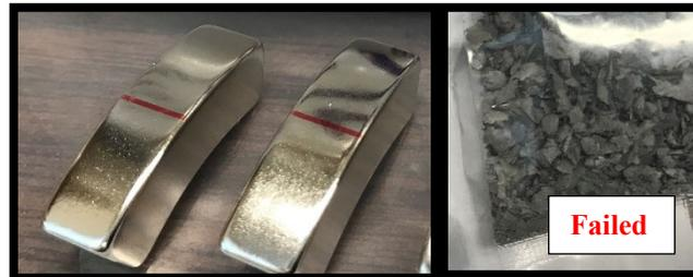
Figure 6. Photo of Magnets Before (left) and After (right; Failed) Testing in a Pressurized Hydrogen Gas Environment
