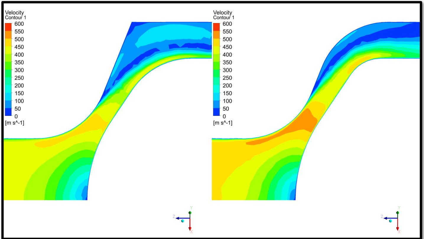
Figure 9. Discharge Valve CFD Velocity Contour Plots for Initial (left) and Final (right) Valve Designs
