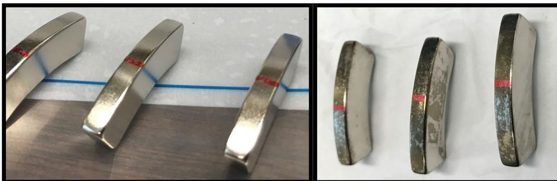
Figure 7. Photo of Magnets Before and After Surviving Testing in a Pressurized Hydrogen Gas Environment
