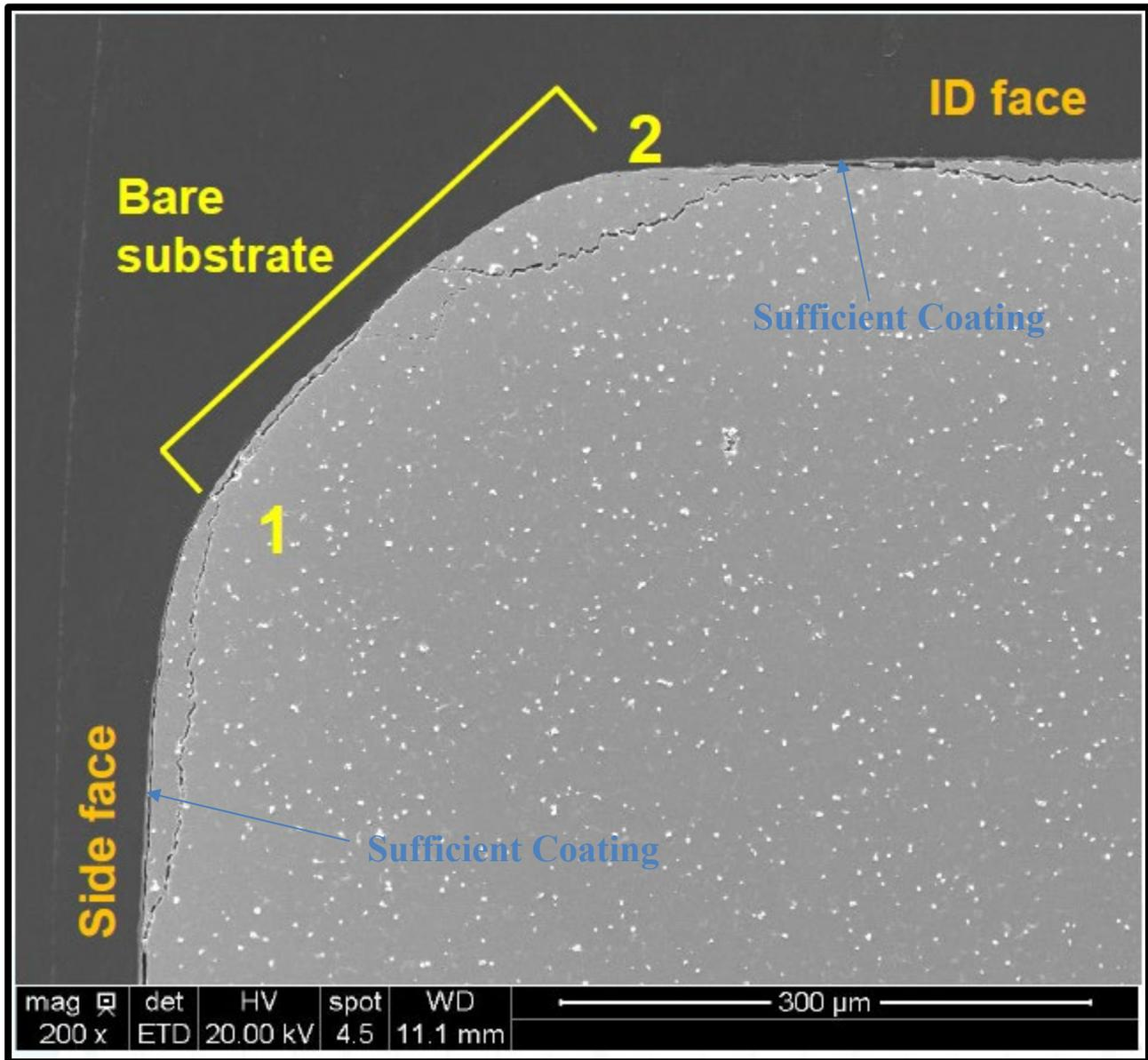
Figure 3. Magnified Image of Sectioned Magnet to Show Missing Coating (Bare Substrate)
