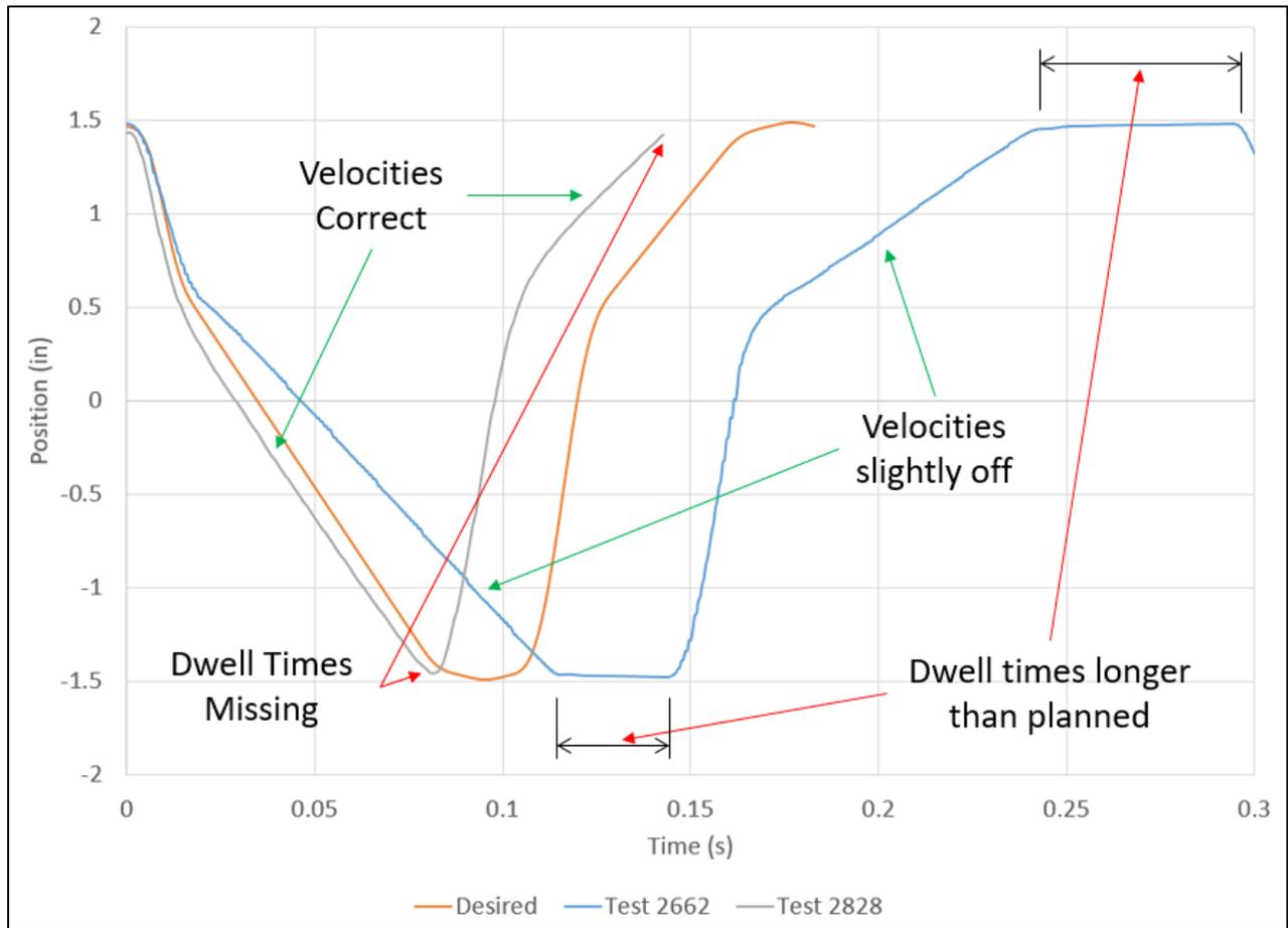
Figure 12. Comparison of Desired to Actual Operating Motion Profiles
