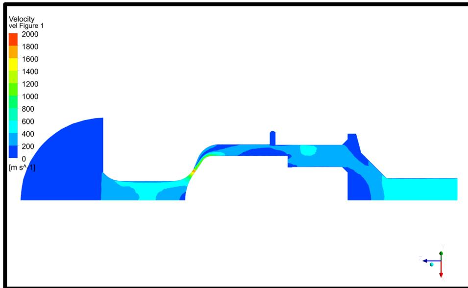
Figure 10. Predicted Velocity Flow Contour for Final Discharge Valve
