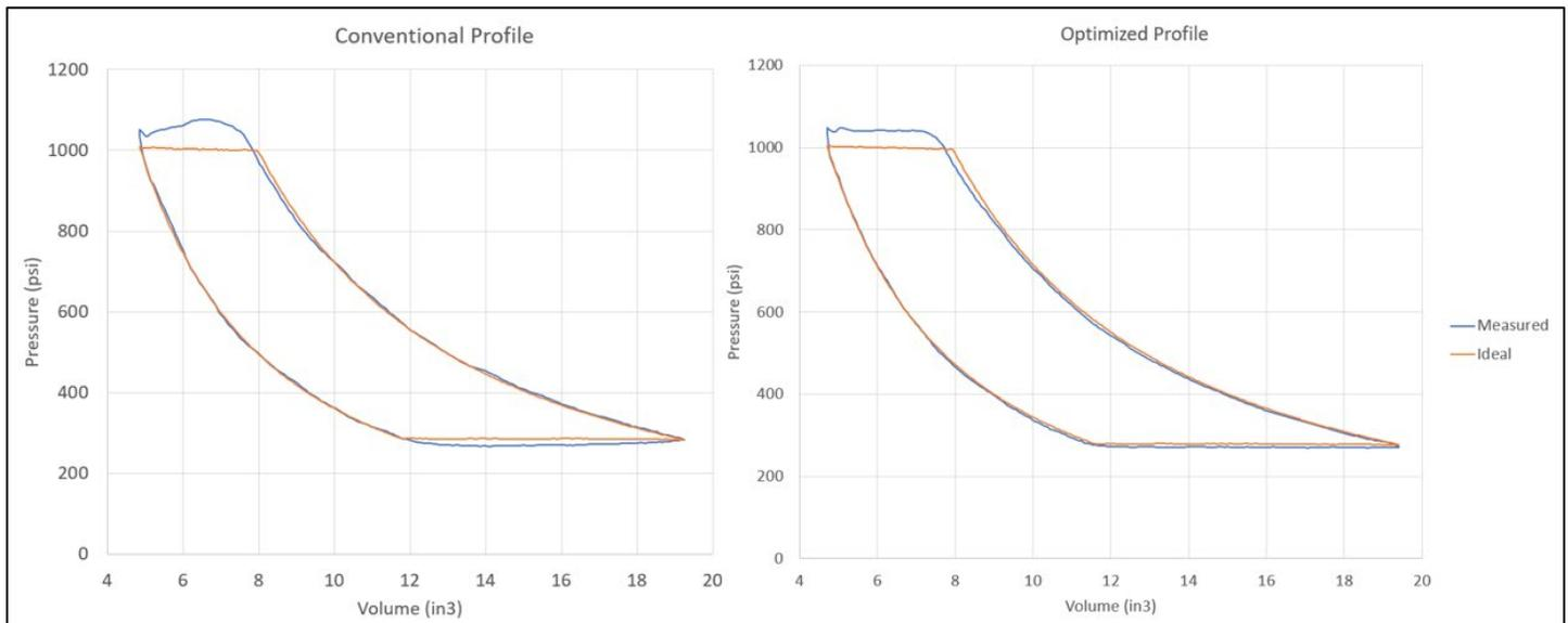
Figure 13. Comparison of Conventional and Optimized Profile Performances
