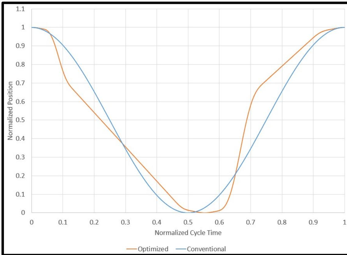
Figure 11. Comparison of Optimized to Conventional Reciprocating Motion Profiles
