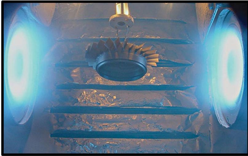
*Figure 4. Image of the plasma enhanced magnetron sputtering (PEMS) process for depositing refractory coatings*
