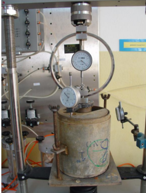
Figura 23. California Bearing Ratio (CBR). Fuente: Jaritngam et al. (57).
