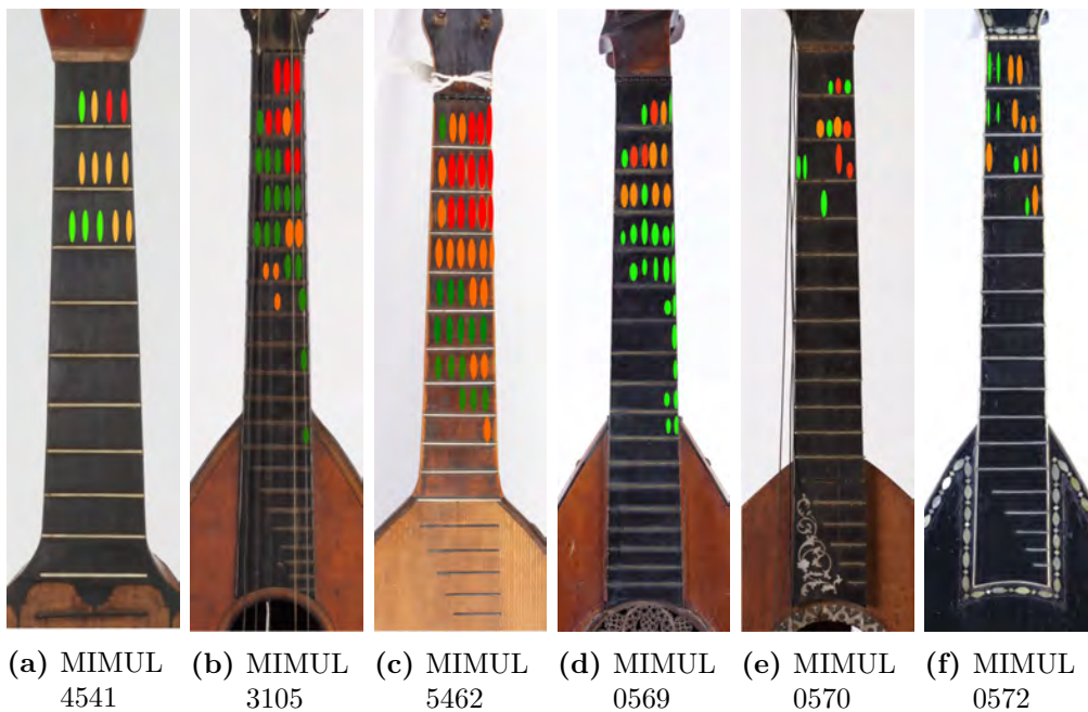
Figure 5.20: Fingerboard wear. Green: light wear, orange: medium, red: heavy
